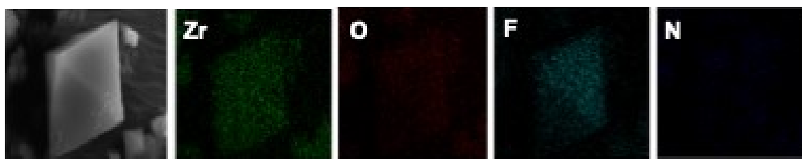
Fig. S11. SEM image and the corresponding energy-dispersive X-ray spectroscopy elemental mapping of UiO-67-CF 3 -50.
