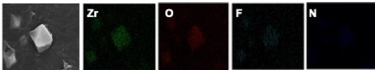
Fig. S12. SEM image and the corresponding energy-dispersive X-ray spectroscopy elemental mapping of UiO-67-CF 3 -25.
