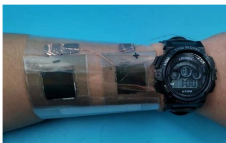
Figure S20. Digital image of a transparent cells under bending state for powering an electronic watch.
