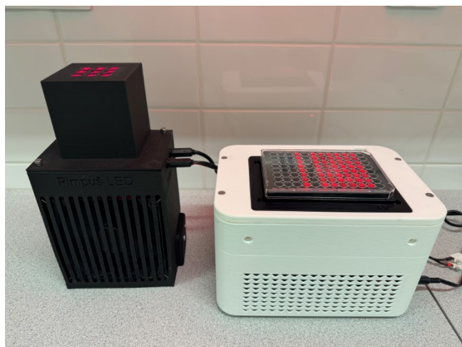
Fig. 9: Custom LED illumination setups (left) configuration for Eppendorf tubes using 656nm LED, (right) configuration for 96-well plates using 625nm LEDs
