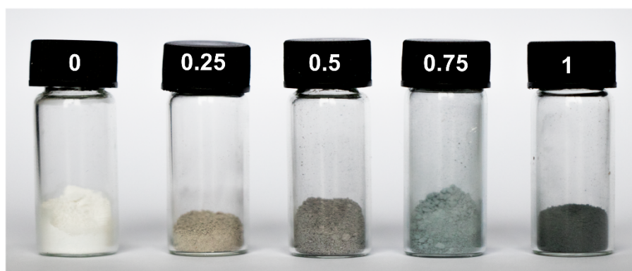
Fig. S1 Photos of \text{TiO}_2 and \text{NaBH}_4 -treated \text{TiO}_2 nanocrystals as a function of weight ratio of \text{NaBH}_4/\text{TiO}_2 .
