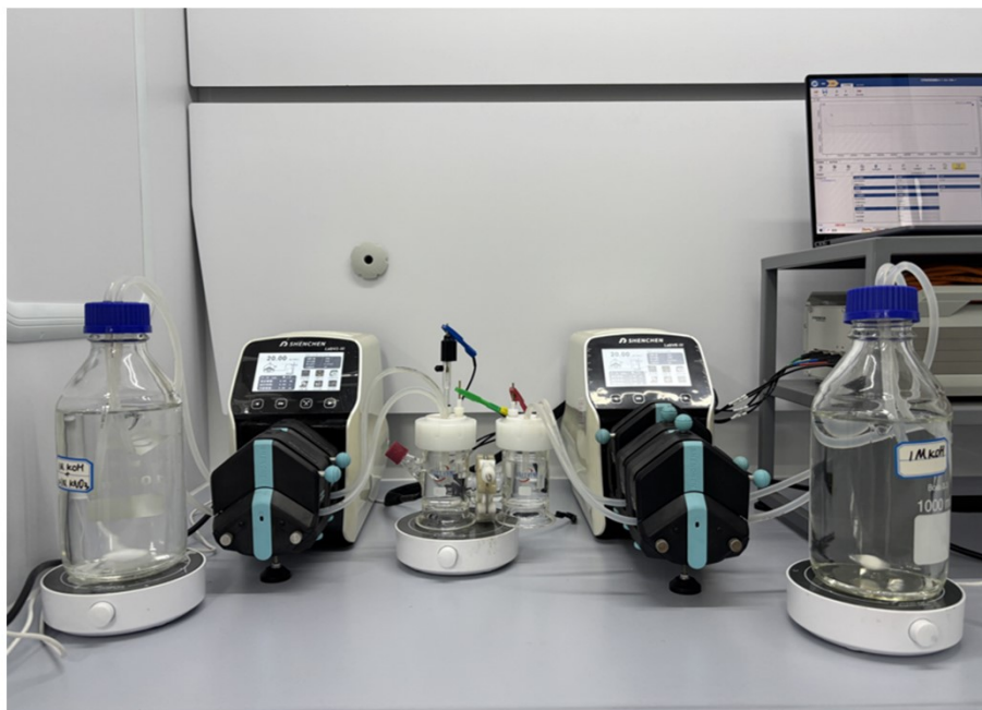
Fig. S23 Schematic illustration of the H-type electrochemical flow cell setup.
