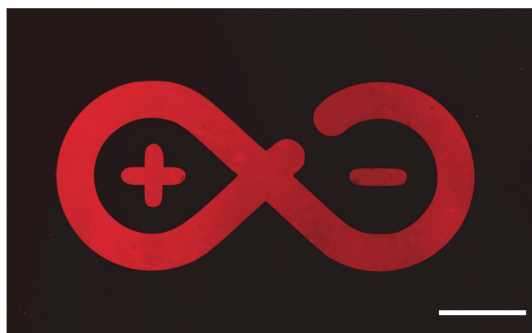
Fig. S14. Fluorescent images of patterns made by red-emitting InP/ZnSe/ZnS QDs. Scale bar, 100 \mu\text{m} .
