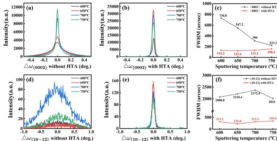
Fig. S5 XRD results of 200 nm AlN films sputtered at different temperatures (600°C, 650°C, 700°C, 750°C).
