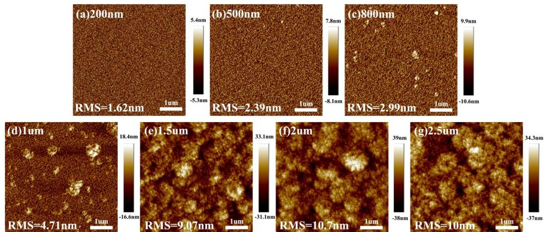
**Fig. S2** AFM results of samples with different thicknesses. (a-g) Films with thicknesses of 200nm, 500nm, 800nm, 1  $\mu$ m, 1.5  $\mu$ m, 2  $\mu$ m, and 2.5  $\mu$ m, respectively.
