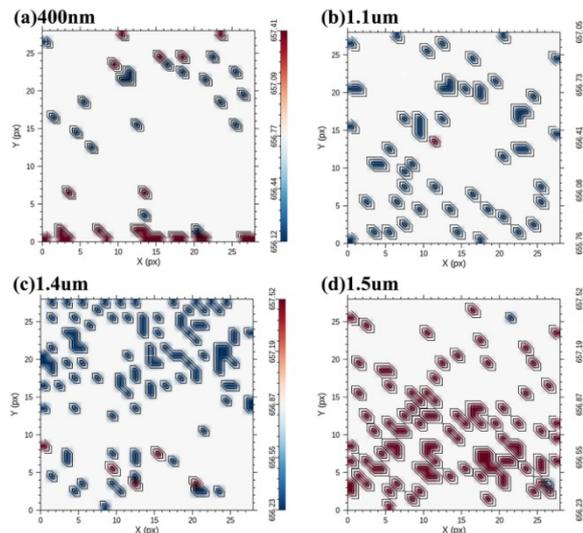
**Fig. S3** Raman mapping of samples with different thicknesses. (a-d) Films with thicknesses of 400 nm, 1.1  $\mu\text{m}$ , 1.4  $\mu\text{m}$ , and 1.5  $\mu\text{m}$ , respectively
