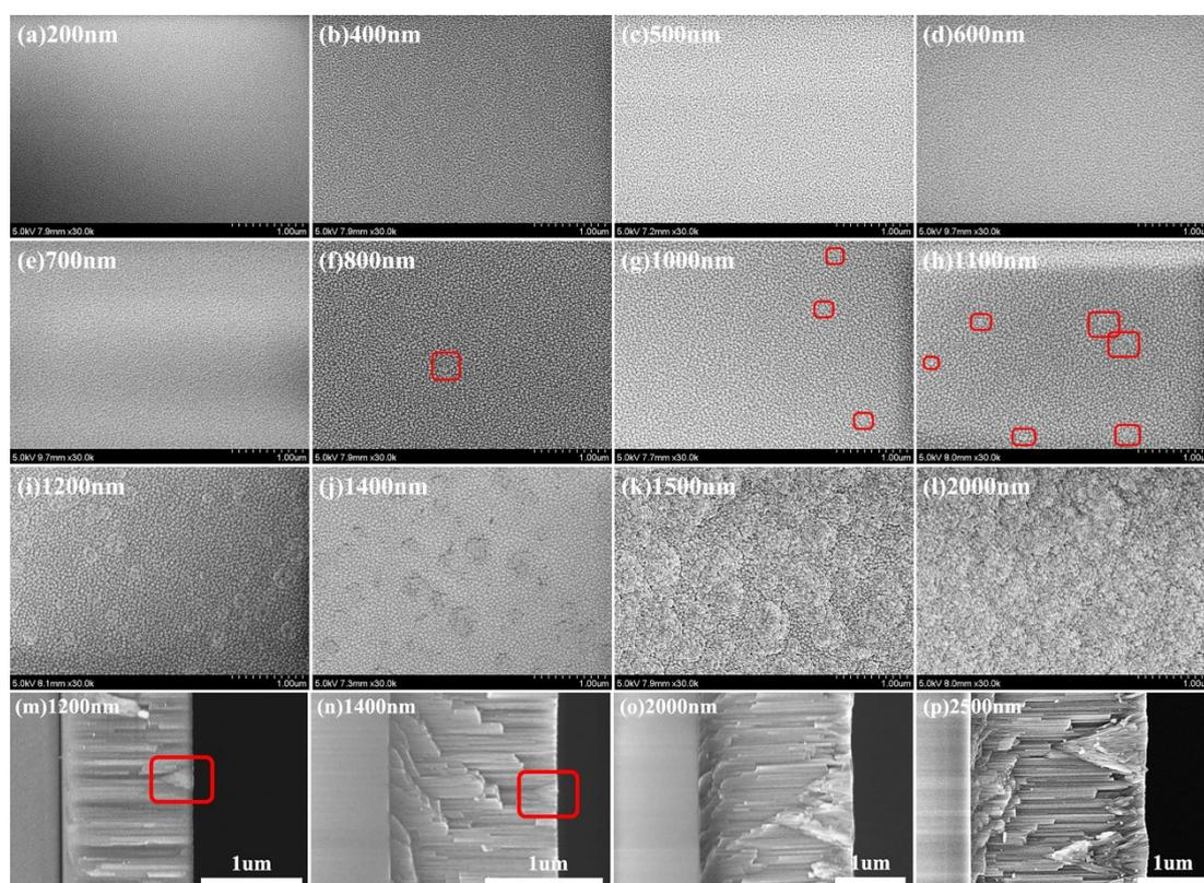
**Fig. S4** SEM results of samples with varying thickness across different batches. (a-l) Surface morphology of the films with thicknesses of 200 nm, 400 nm, 500 nm, 600 nm, 800 nm, 1  $\mu\text{m}$ , 1.1  $\mu\text{m}$ , 1.2  $\mu\text{m}$ , 1.4  $\mu\text{m}$ , 1.5  $\mu\text{m}$  and 2  $\mu\text{m}$ , respectively. (m-p) Cross-sectional of the films with thicknesses of 1.2  $\mu\text{m}$ , 1.4  $\mu\text{m}$ , 2  $\mu\text{m}$  and 2.5  $\mu\text{m}$ , respectively.
