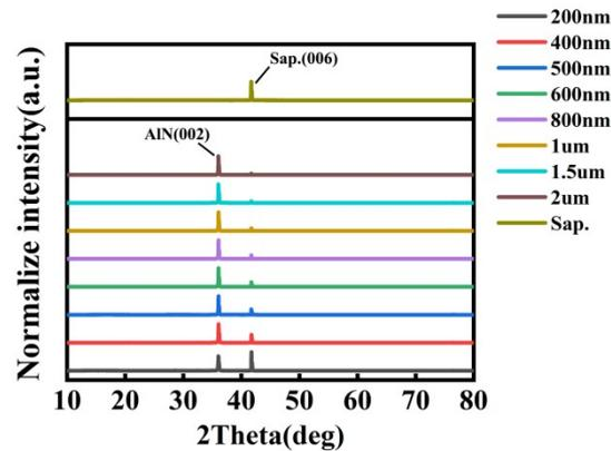
**Fig. S1** XRD 2Theta-Omega test of a wide range ( $10^{\circ}$ – $80^{\circ}$ ) on samples with different thicknesses and sapphire substrate.
