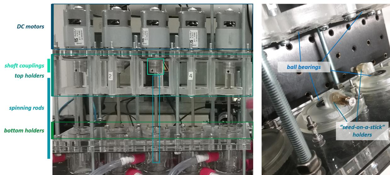
Figure S2: **left:** Picture of the motor platform unit. This rigid construction eliminates eccentricity and ensures reproducible positioning of the overhead stirrers. **right:** Close-up of the bottom 3D printed holder, highlighting holders where the “seed-on-a-stick” can be inserted and secured.
