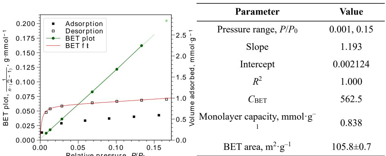
Figure S9. BET surface area calculations for **1a** based on carbon dioxide adsorption isotherm at 195 K.
