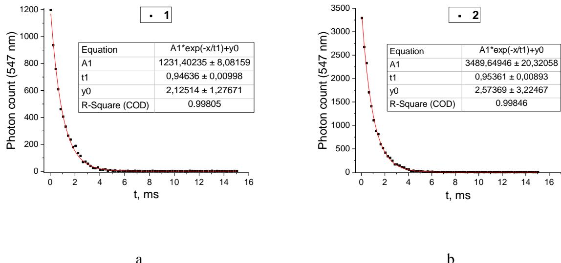
Figure S12. Phosphorescence decay fitting curves for **1** (a) and **2** (b)
