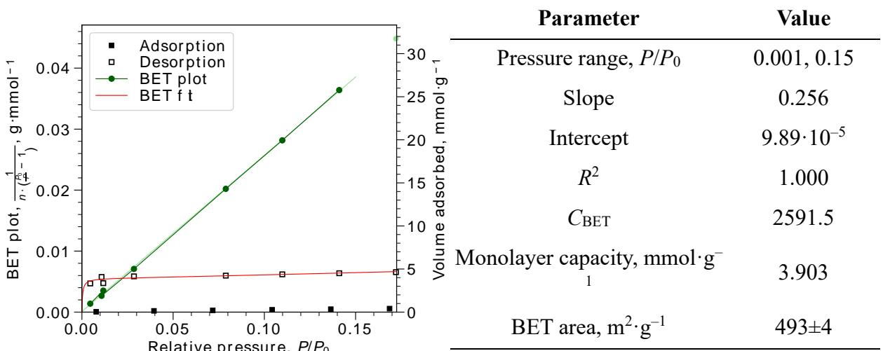
Figure S8. BET surface area calculations for **2a** based on carbon dioxide adsorption isotherm at 195 K.
