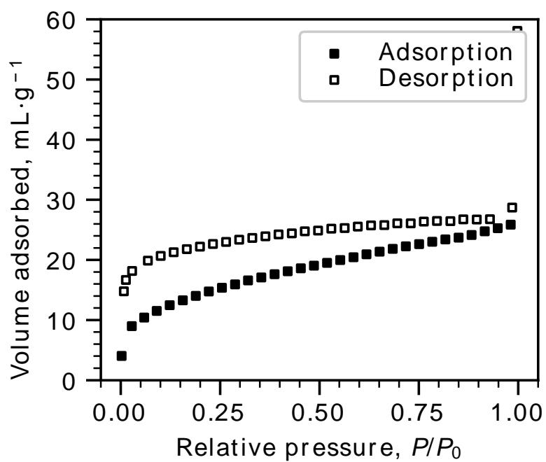
Figure S7. CO<sub>2</sub> adsorption-desorption isotherm for the sample **1a** at 195 K.
