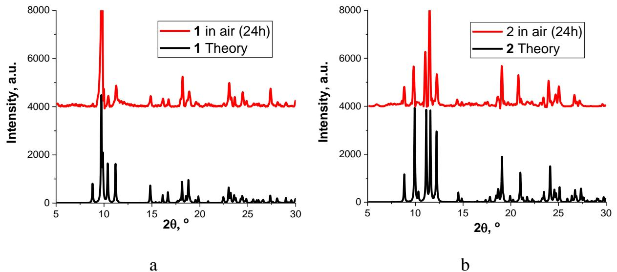
Figure S3. PXRD patterns for the polycrystalline powders of **1** and **2** after 24h storage in air.
