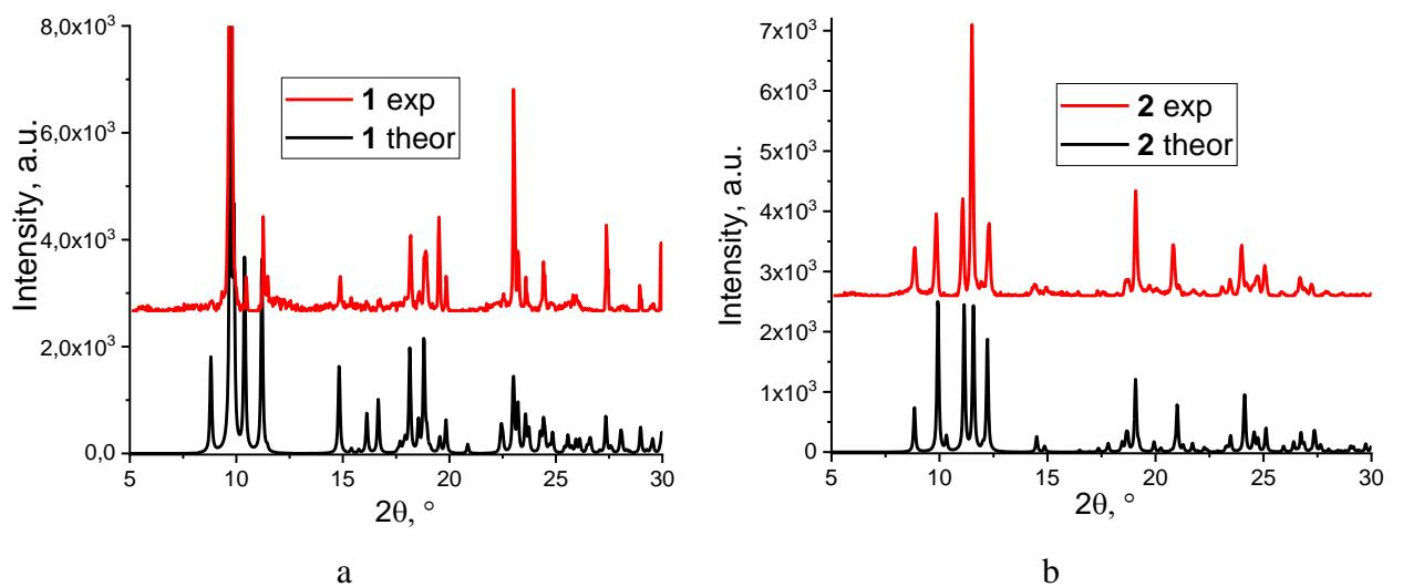
Figure S1. PXRD patterns for **1** (a) and **2** (b) compared to the theoretical ones.
