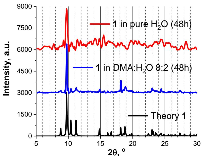
Figure S4. PXRD patterns for the polycrystalline powders of **1** after 48h storage in  $\text{H}_2\text{O}$  or DMA- $\text{H}_2\text{O}$  mixture.
