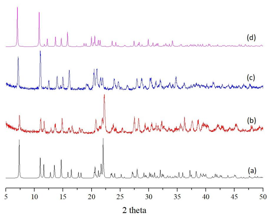
**Fig. S16.** (a) Simulated PXRD pattern of **9**, (b) as-synthesized PXRD pattern of **9**, (c) PXRD pattern of the sample of (b) heated in water at  $140\text{ }^\circ\text{C}$  for 2 days and (d) simulated PXRD pattern of **10**.
