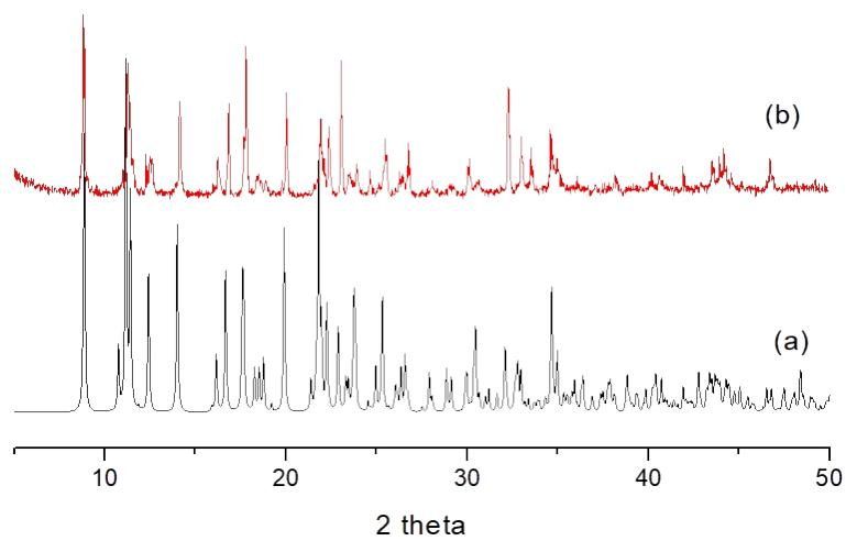
**Fig. S8.** (a) Simulated and (b) experimental PXRD patterns of **5**.
