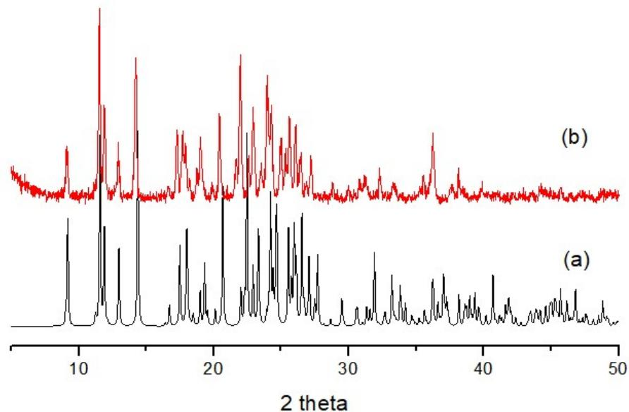
**Fig. S6.** (a) Simulated and (b) experimental PXRD patterns of **3**.
