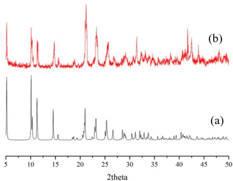
**Fig. 10.** (a) Simulated and (b) experimental PXRD patterns of 7.
