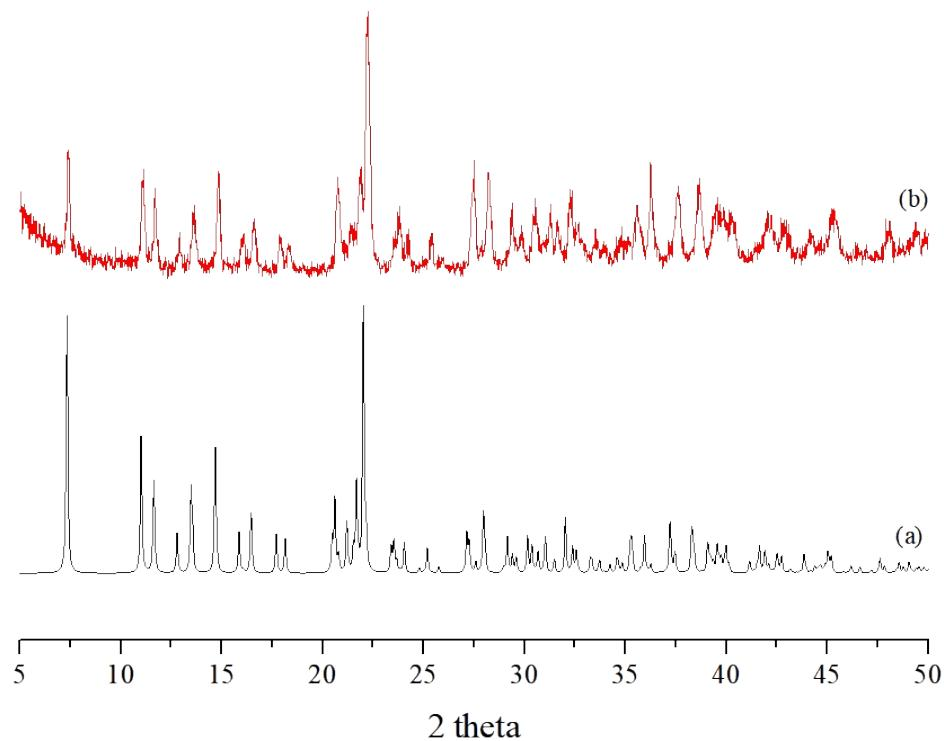
**Fig. S13.** (a) Simulated and (b) experimental PXRD patterns for **10**.
