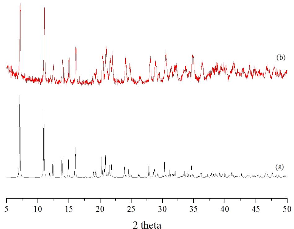
**Fig. S14.** (a) Simulated and (b) experimental PXRD patterns for **11**.
