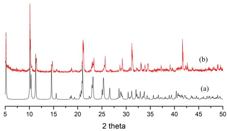
**Fig. 9.** (a) Simulated and (b) experimental PXRD patterns of **6**.
