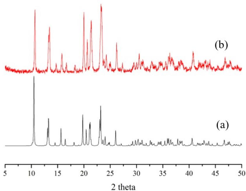
**Fig. S11.** (a) Simulated and (b) experimental PXRD patterns for **8**.
