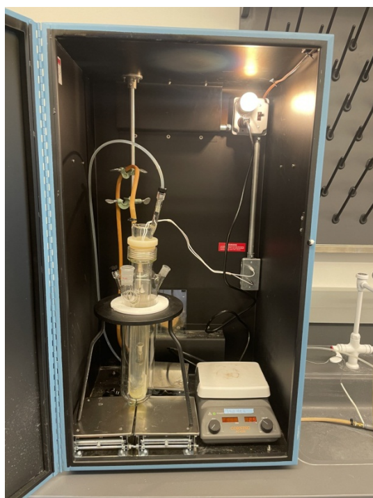
Figure S2. Experimental setup to expose (4,6-diCl res)·2(PEB) to heat and ultraviolet light simultaneously within the photoreactor.
