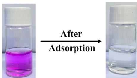
Figure S17. The optical image of the MnO 4 - solution before and after removal by DPOC-1.
