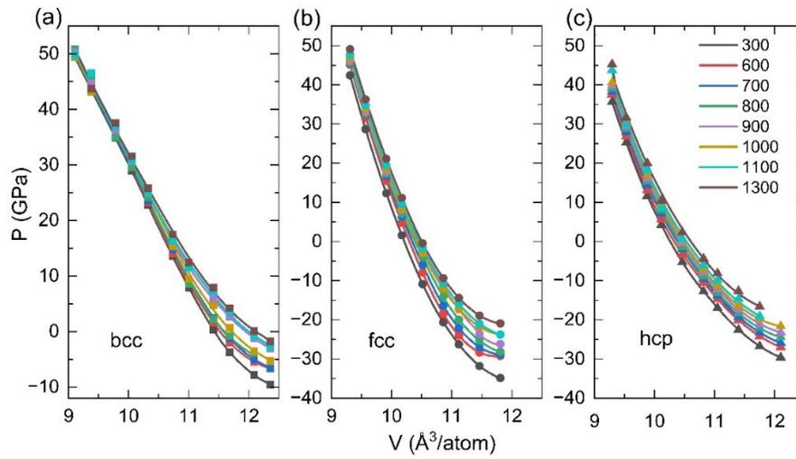
**Figure S6** Pressure-volume relation obtained from FFMD of Fe for bcc phase (a), fcc phase (b), and hcp phase (c), respectively.
