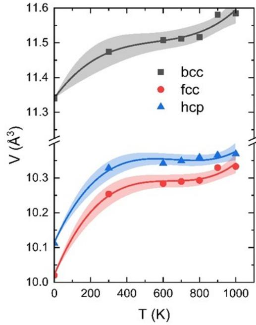
**Figure S7** Volume-temperature relation obtained from FFMD of Fe for bcc phase, fcc phase, and hcp phase, respectively.
