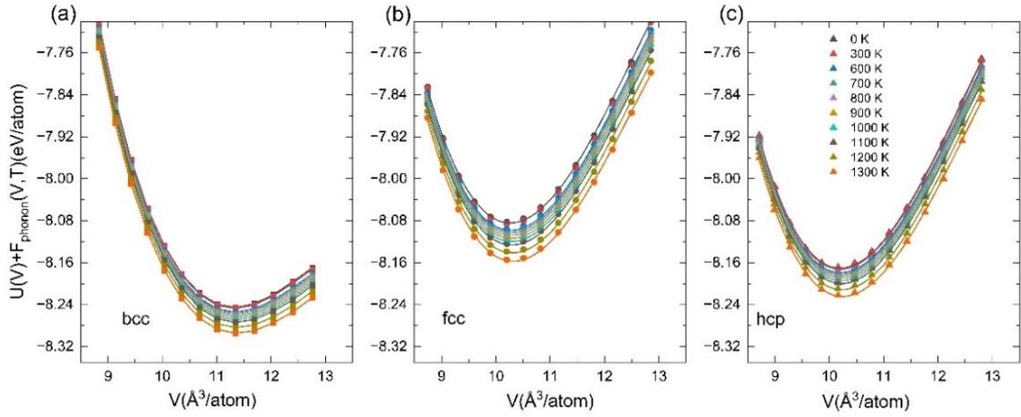
**Figure S5** Free energy  $F(V, T)$  versus volumes of Fe for bcc (solid line), fcc (dotted line), and hcp (dashed line) phases at different temperatures through the QHA method.
