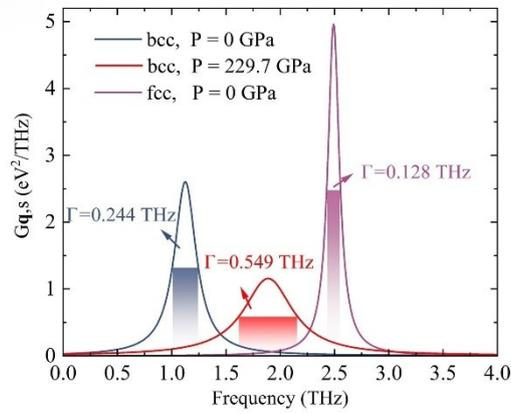
**Figure S10** The power spectrum  $G_{q,s}$  and linewidth  $\Gamma$ . Note that the blue, red, and purple lines are for 0 GPa bcc, 229.7 GPa bcc, and 0 GPa fcc Fe, respectively. The calculation temperature is 300 K.
