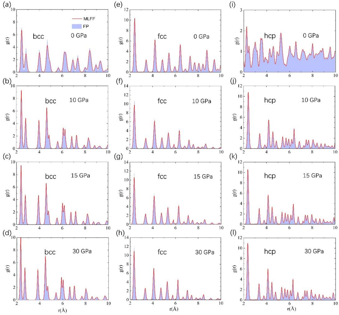
**Figure S2** The pair correlation function of (a-d) bcc, (e-h) fcc, and (i-l) hcp phase of iron obtained by AIMD and FFMD. The purple area is the AIMD calculation results and the red line is the FFMD results.
