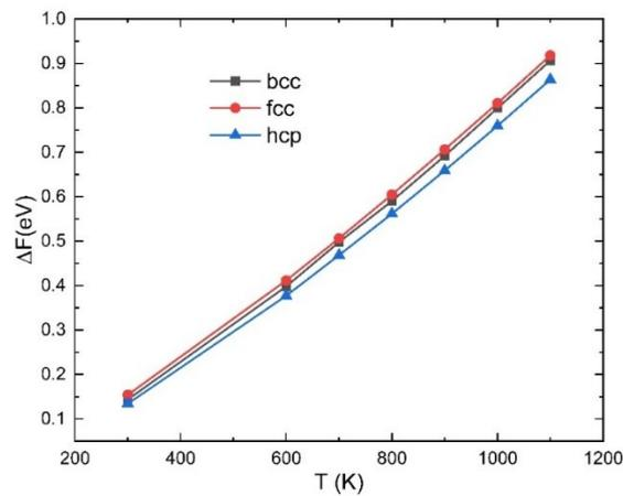
**Figure S11** The energy difference  $\Delta F = -T(S_{\text{anharm}} - S_{\text{harm}})$  of bcc, fcc, and hcp phase of Fe as a function of temperature at  $V_{\text{eq}}$  ( $T=0\text{K}$ ).
