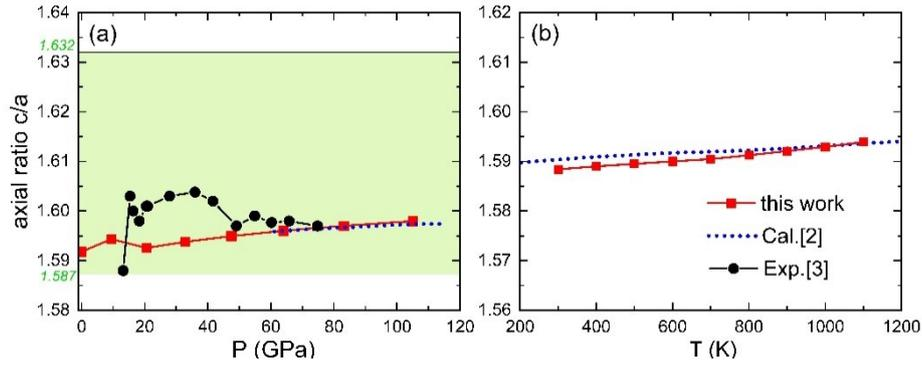
**Figure S4** The  $c/a$  ratio of hcp Fe at different pressures and temperatures. The green shaded area in (a) was obtained from [1]. The red lines are the results of the calculations in this paper, the blue dotted line is the reference of the theoretical calculations [2], and the red data is the experimental values [3]. Note that (a) was calculated at 300 K and 0 GPa.
