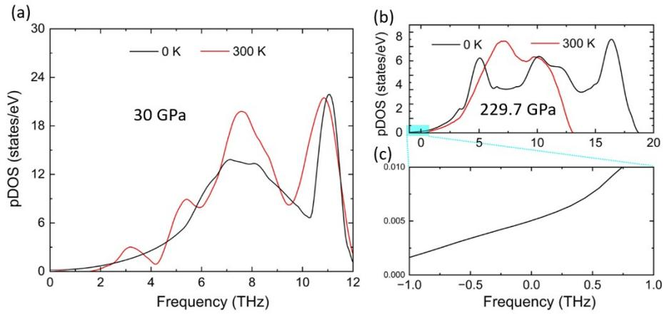
**Figure S9** The calculated phonon density of states (pDOS) of bcc at 30 GPa and 229.7 GPa, respectively. The black line and red line were calculated at 0 K and 300 K, respectively.
