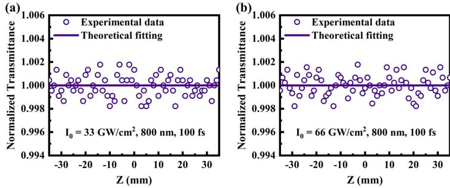
**Fig. S2.** Open-aperture Z-scan curves for clean fused quartz at low incident light intensities of (a) 33  $\text{GW/cm}^2$  and (b) 66  $\text{GW/cm}^2$ .
