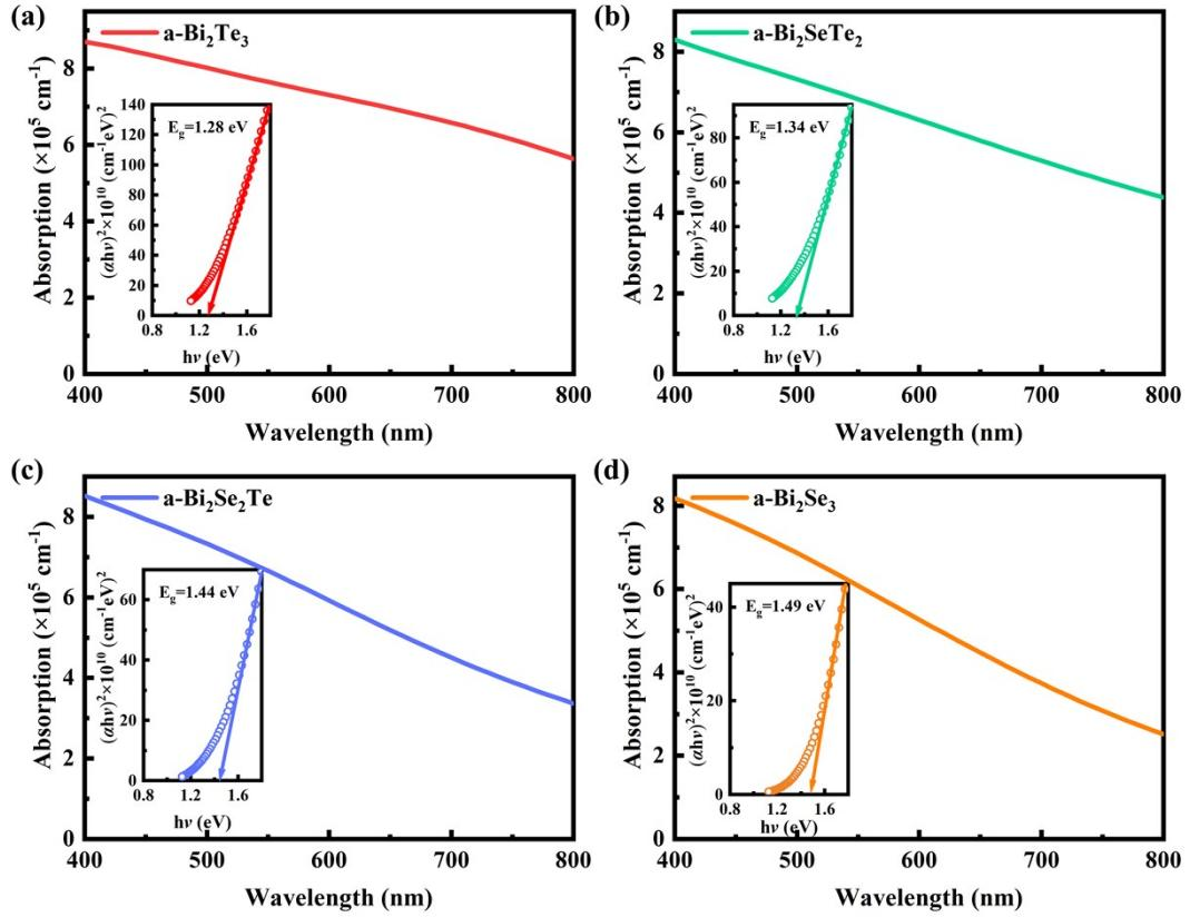
**Fig. S1.** Absorption coefficient spectra and Tauc plots (insets) of a-Bi<sub>2</sub>Se<sub>x</sub>Te<sub>3-x</sub> thin films: (a) a-Bi<sub>2</sub>Te<sub>3</sub>, (b) a-Bi<sub>2</sub>SeTe<sub>2</sub> (c) a-Bi<sub>2</sub>Se<sub>2</sub>Te, (d) a-Bi<sub>2</sub>Se<sub>3</sub>.
