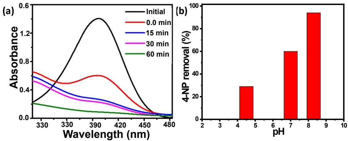
**Figure S7.** (a) UV–vis spectra for photodegradation of 20 ppm 4-NP in aqueous medium of pH 8.3 using catalyst 0.2 AC-MMO under Xe lamp irradiation, (b) Histogram of degradation of 4-NP under various pH conditions. (Note: The pH of 4-NP solution is varied by the addition of HCl and NaOH.)
