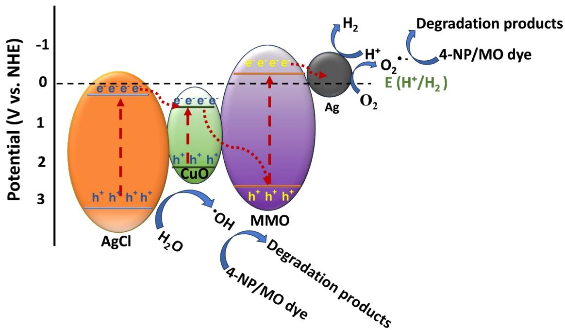
**Figure S9.** Proposed mechanism for UV-visible-light-induced photocatalytic reaction over the 0.2AC-MMO photocatalyst.
