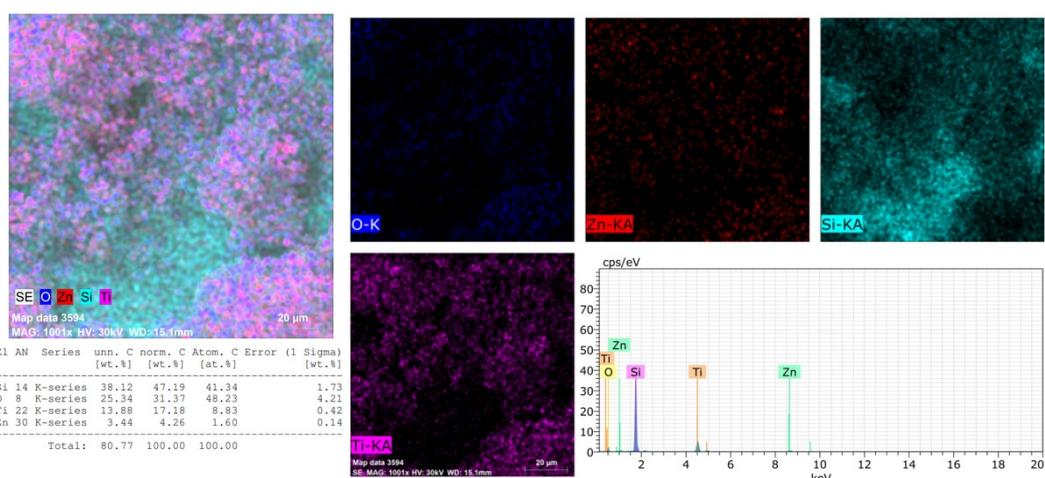
**Figure S2.** EDS and elemental mapping for MMO
