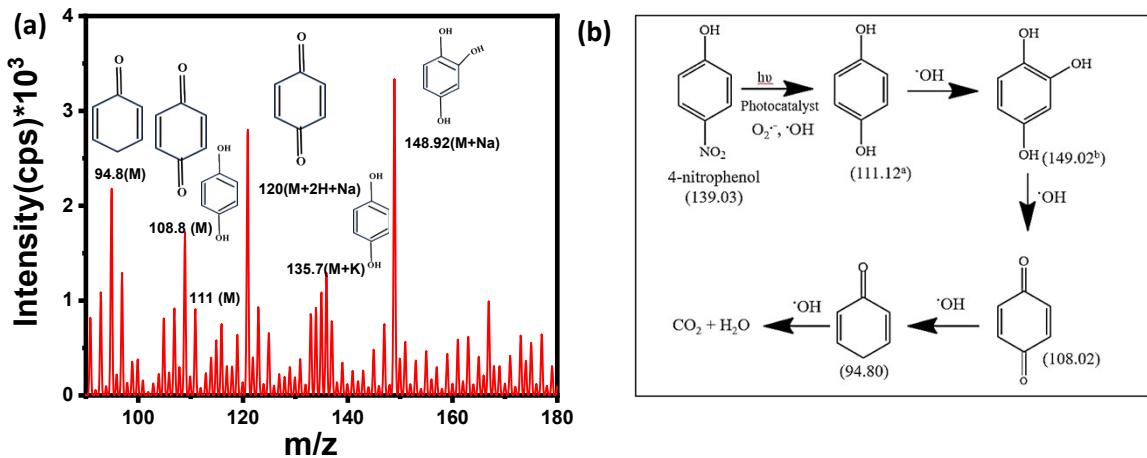
**Figure S8.** (a) LC-MS analysis of 4-NP degradation after 1h light irradiation (broad-spectrum), (b) Schematic depiction of the process involved in the degradation of 4-NP. The proposed degradation pathways via photogenerated species of photodegraded 4-nitrophenol (the corresponding m/z value of different intermediates identified by LC-MS).
