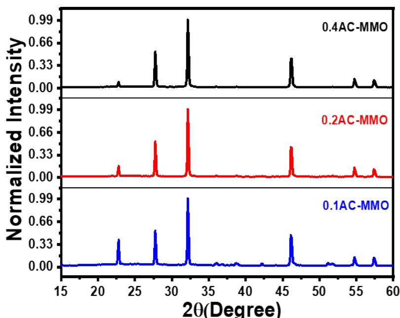
**Figure S1.** XRD pattern of synthesized AC-MMO using different molar ratios of  $\text{AgNO}_3$  reaction on  $\text{CuO}/\text{MMO}$ .
