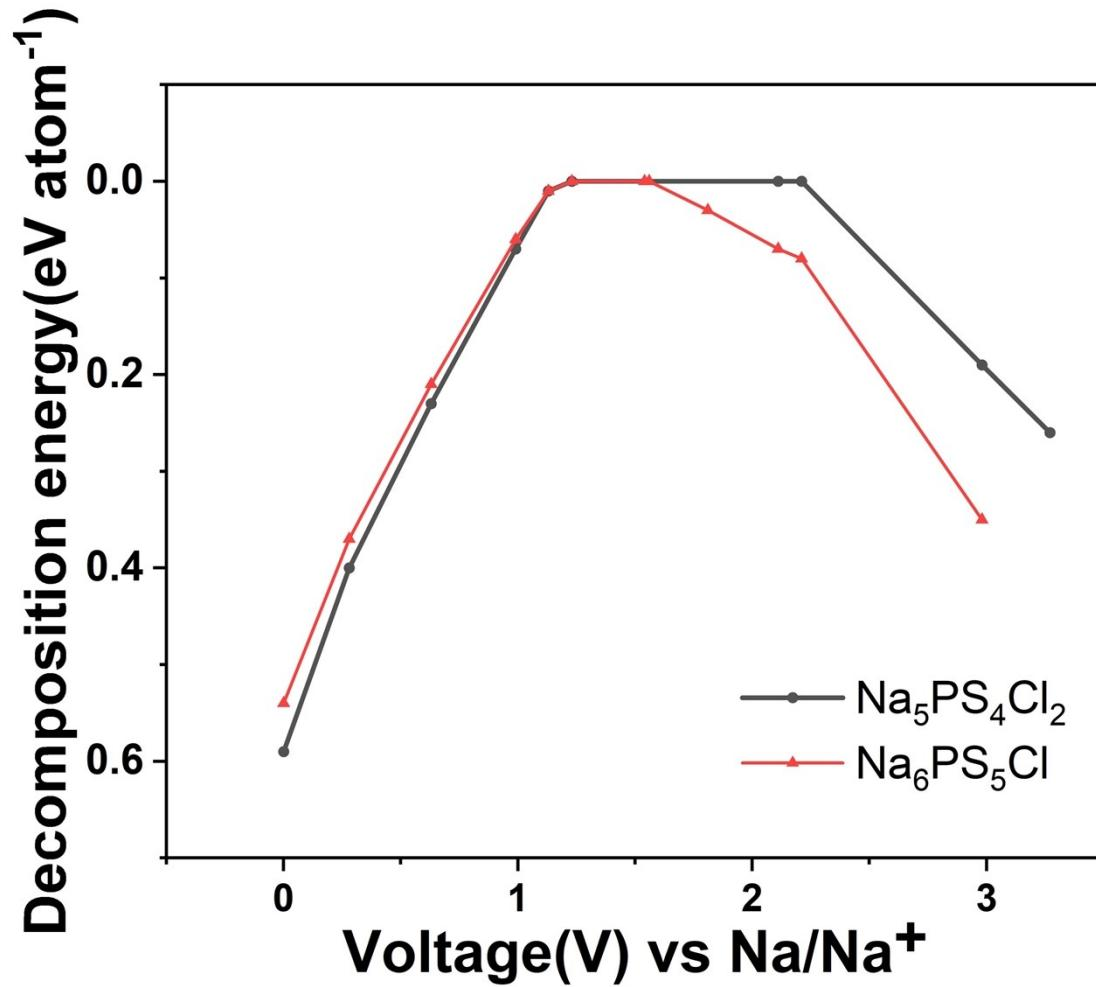
**Fig. S10** The decomposition energy of NPSC1 and NPSC2as a function of the chemical potential of Na-ions.
