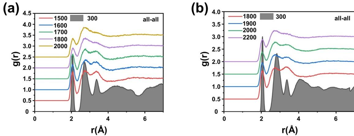
**Fig. S4** The radial distribution function of all-all in (a) NPSC1, and (b) NPSC2
