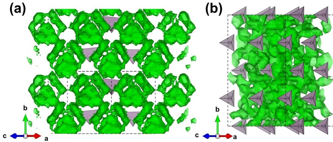
**Fig. S7** The Na-ions probability density superimposed (green) on the anion sublattice of NPSC1 (1000 K) and NPSC2 (1300 K), the data from AIMD simulations.
