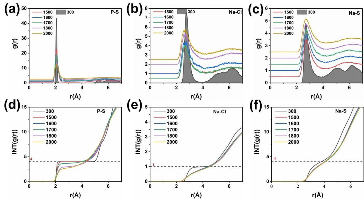
**Fig S5** (a-c) The radial distribution function of P-S, Na-Cl, and Na-S in NPSC1. (d-f) The integral of the radial distribution function of P-S, Na-Cl, and Na-S in NPSC1.
