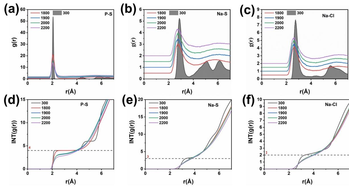
**Fig S6** (a-c) The radial distribution function of P-S, Na-Cl, and Na-S in NPSC2. (d-f) The integral of the radial distribution function of P-S, Na-Cl, and Na-S in NPSC2.
