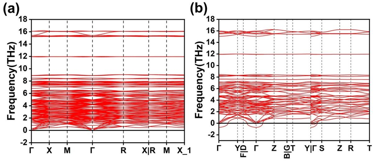
**Fig. S2** The phonon spectra of (a) NPSC1, and (b) NPSC2.
