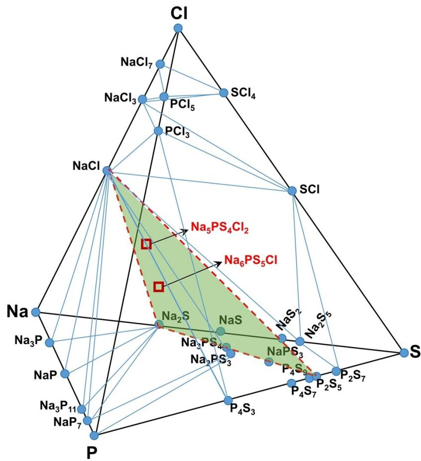
**Fig. S1** Na-P-S-Cl Four-Component Phase Diagram.
