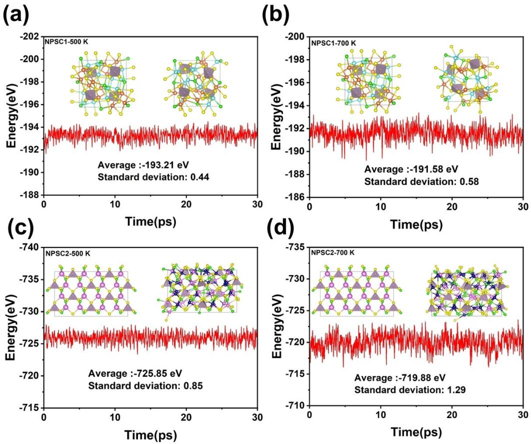
**Fig. S3** Total energy fluctuation during the AIMD simulations at 500 K and 700 K of (a) NPSC1, and (b) NPSC2.
