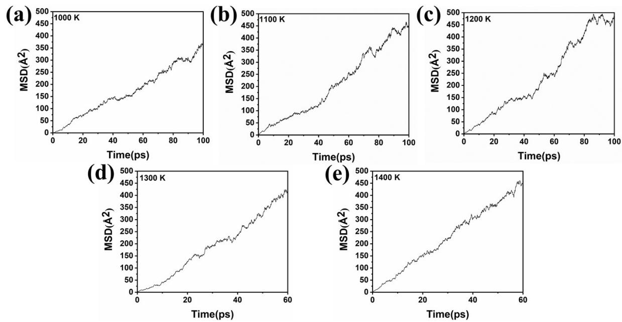
**Fig. S8** MSD plots of NPSC1 for AIMD simulations. (a) 100ps AIMD simulation at 1000K. (b) 100ps AIMD simulation at 1100K. (c) 100ps AIMD simulation at 1200K. (d) 60ps AIMD simulation at 1300K. (e) 60ps AIMD simulation at 1400K.
