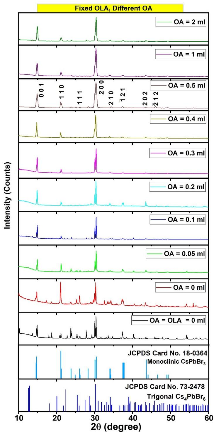
**Fig. S11** XRD patterns of CsPbBr<sub>3</sub> NCs prepared with a fixed OLA and varying OA concentration.
