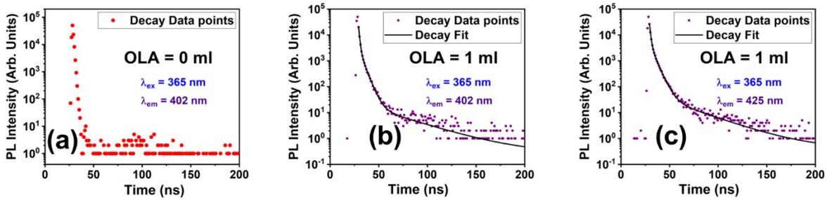
**Fig. S6** PL decay curves for the blue emissions of CsPbBr<sub>3</sub> NCs excited at 365 nm showing the variation of the decay kinetics for fixed OA concentration and different OLA concentrations: (a) OLA = 0 ml for 402 nm, (b) OLA = 1 ml for 402 nm, and (c) OLA = 1 ml for 426 nm.
