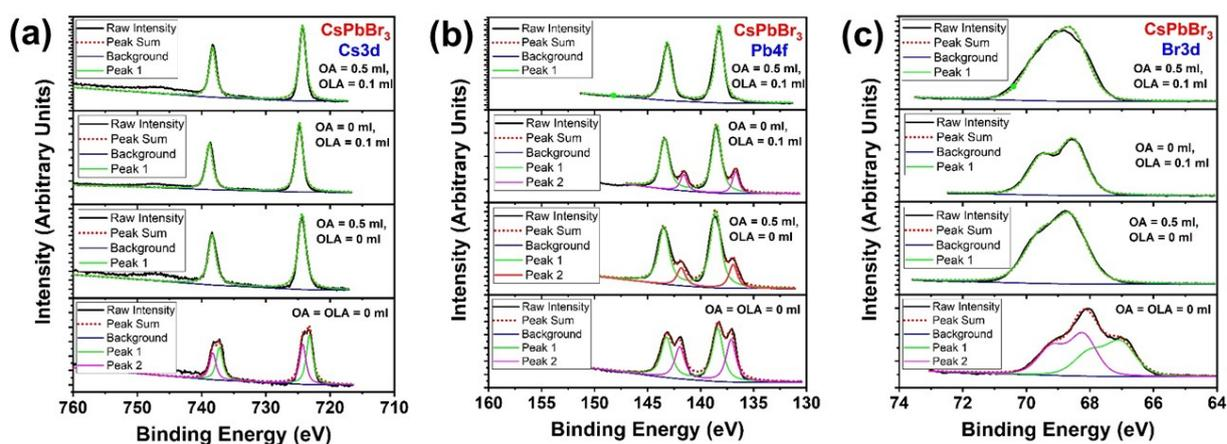
**Fig. S13** High-resolution XPS spectra for (a) Cs 3d, (b) Pb 4f, and (c) Br 3d, for the CsPbBr<sub>3</sub> samples prepared without adding any ligands, prepared by adding either OA or OLA, and prepared using the optimized quantities of both OA and OLA.
