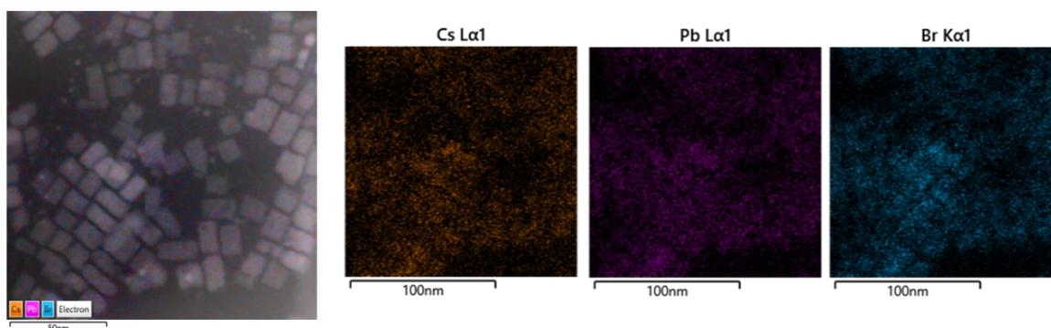
**Fig. S9** Elemental map obtained from the EDS showing the distribution of the constituent elements in CsPbBr<sub>3</sub> NCs prepared using the optimized quantities of both OA and OLA.
