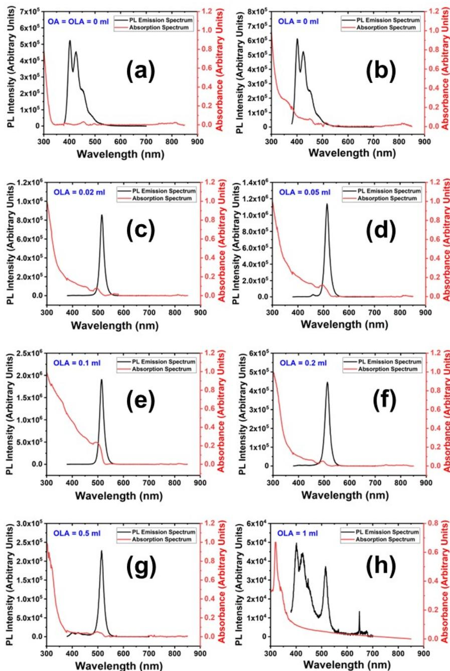
**Fig. S1** UV-Visible absorbance and PL emission spectra of CsPbBr<sub>3</sub> NCs. (a) NCs prepared without using OA or OLA during the synthesis. (b-h) NCs prepared with a fixed amount of OA (0.5 ml) and varying amounts of OLA ranging from 0 to 1 ml: (b) OLA = 0 ml, (c) OLA = 0.02 ml, (d) OLA = 0.05 ml, (e) OLA = 0.1 ml, (f) OLA = 0.2 ml, (g) OLA = 0.5 ml, and (h) OLA = 1 ml.
