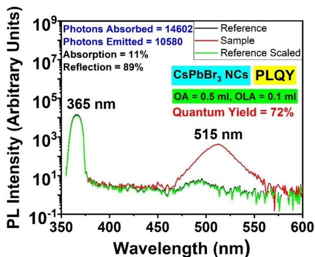
**Fig. S5** Emission spectra for the determination of PLQY for CsPbBr<sub>3</sub> NCs prepared using 0.5 ml OA and 0.1 ml OLA.
