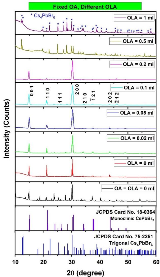
**Fig. S10** XRD patterns of  $\text{CsPbBr}_3$  NCs prepared with a fixed OA and varying OLA concentration.
