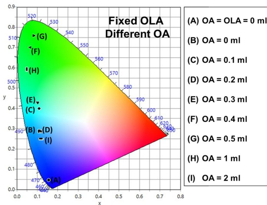
**Fig. S4** CIE 1931 chromaticity diagram showing the variation of color emission from CsPbBr<sub>3</sub> NCs under 365 nm excitation for fixed OLA and varying OA concentrations.
