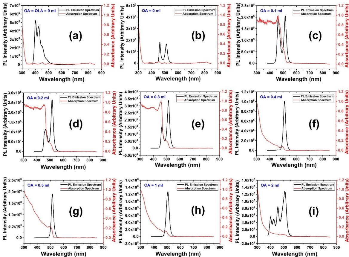
**Fig. S2** UV-Visible absorbance and PL emission spectra of CsPbBr<sub>3</sub> NCs. (a) NCs prepared without using OA or OLA during the synthesis. (b-i) NCs prepared with a fixed amount of OLA (0.1 ml) and varying amounts of OA ranging from 0 to 2 ml: (b) OA = 0 ml, (c) OA = 0.1 ml, (d) OA = 0.2 ml, (e) OA = 0.3 ml, (f) OA = 0.4 ml, (g) OA = 0.5 ml, (h) OA = 1 ml, and (i) OA = 2 ml.
