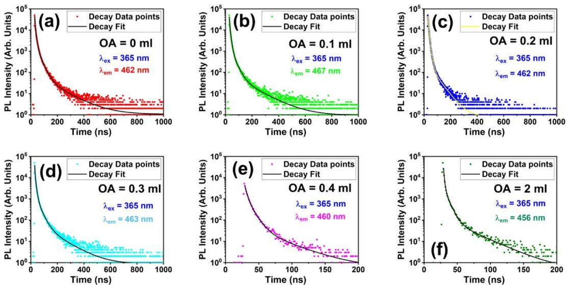
**Fig. S7** PL decay curves for the blue emissions of CsPbBr<sub>3</sub> NCs excited at 365 nm showing the variation of the decay kinetics for fixed OLA concentration and different OA concentrations: (a) OA = 0 ml for 462 nm, (b) OA = 0.1 ml for 467 nm, (c) OA = 0.2 ml for
