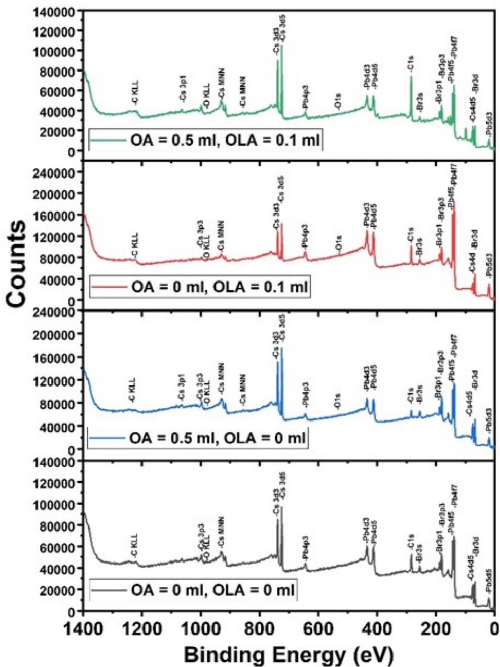
**Fig. S12** XPS full-survey scan for the CsPbBr<sub>3</sub> samples prepared without adding any ligands, prepared by adding either OA or OLA, and prepared using the optimized quantities of both OA and OLA.
