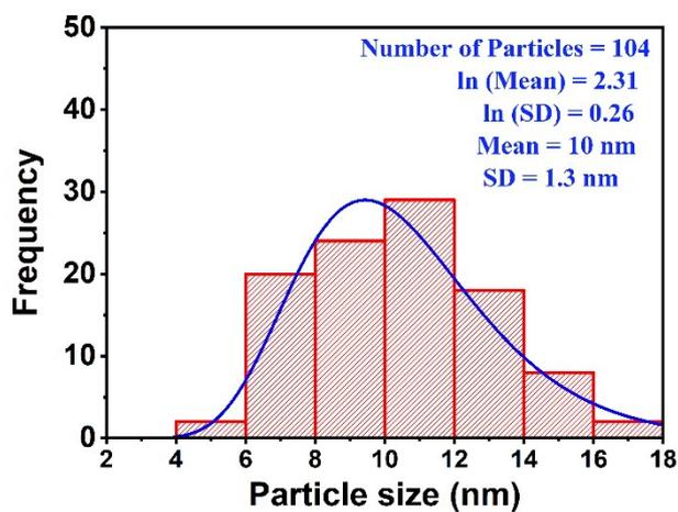
**Fig. S8** Particle-size distribution of the CsPbBr<sub>3</sub> NCs prepared using the optimized quantities of both OA and OLA.
