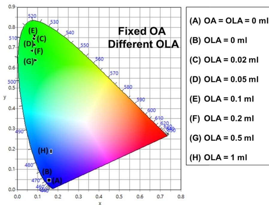
**Fig. S3** CIE 1931 chromaticity diagram showing the variation of color emission from CsPbBr<sub>3</sub> NCs under 365 nm excitation for fixed OA and varying OLA concentrations.
