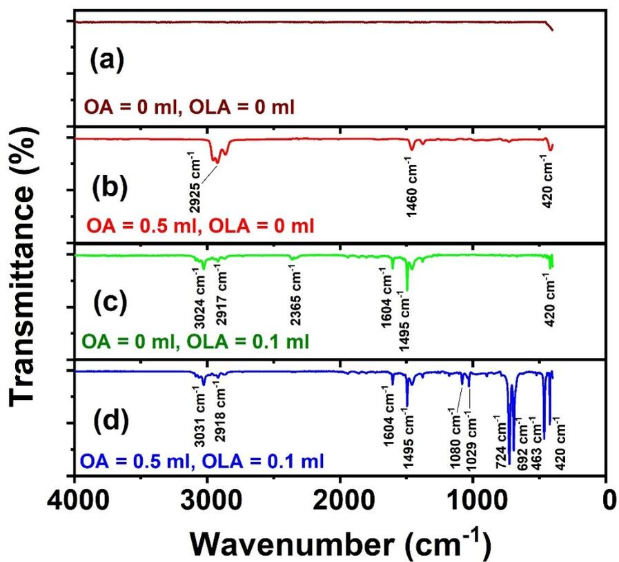
**Fig. S14** FTIR spectra of the CsPbBr<sub>3</sub> NCs prepared: **(a)** without OA or OLA, **(b)** with only OA, **(c)** with only OLA, and **(d)** with both optimized quantities of OA and OLA.
