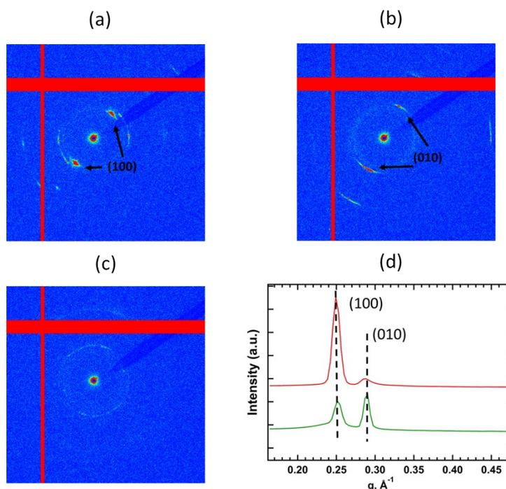
Fig. S2. Selected two-dimensional X-ray scattering patterns recorded from different regions of the M1 sample isothermally crystallized at 123 °C: (a) region with high intensity of the 100 peak, (b) region with high intensity of the 010 peak, and (c) region with low intensity of both peaks. (d) 1D-reduced X-ray scattering data exemplified for samples M1 (red) and M2 (green).
