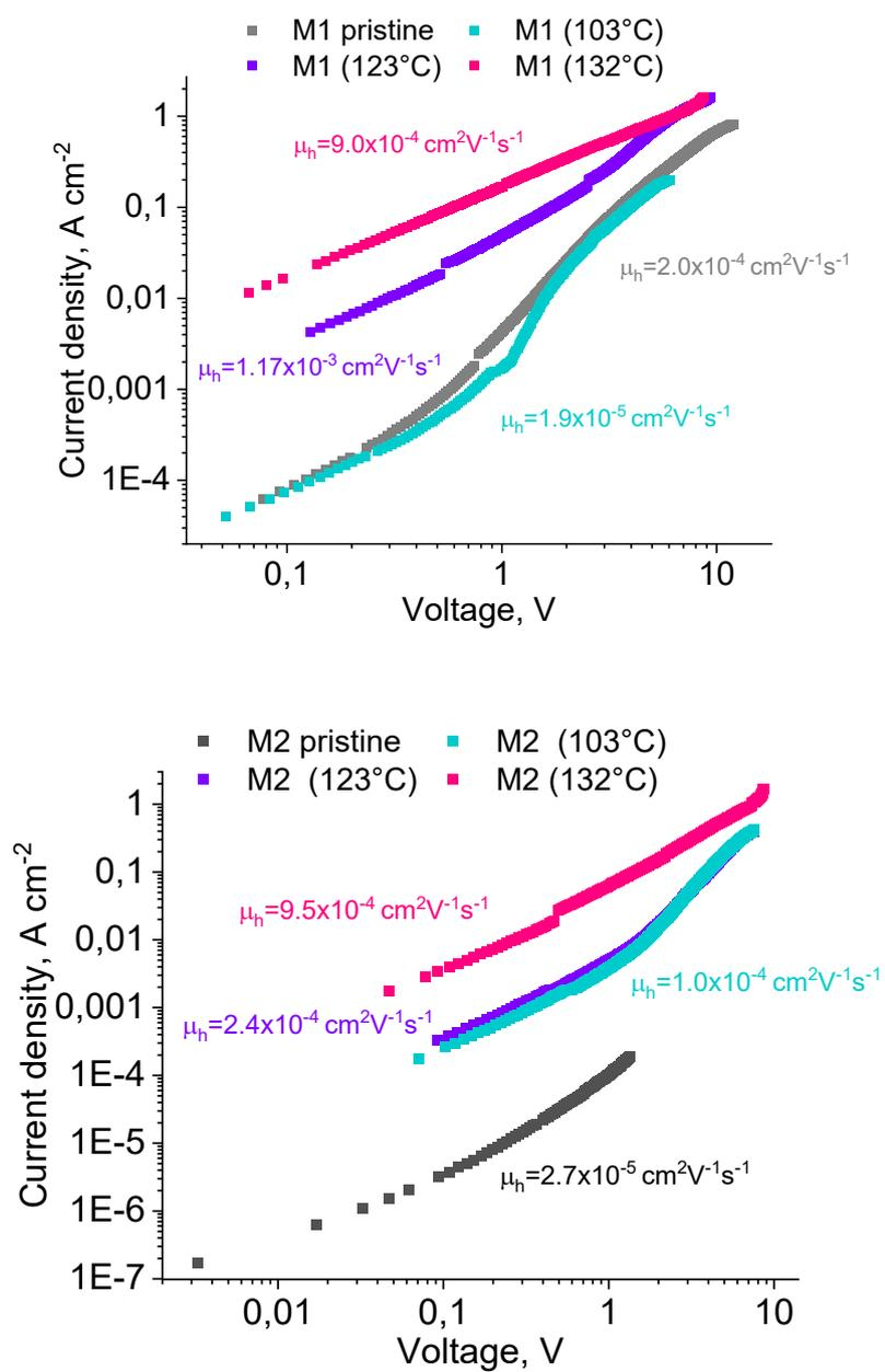
Fig. S4. – J-V curves for hole-only devices with active layers of samples M1 (top panel) and M2 (bottom panel) isothermally crystallized at the indicated temperatures.
