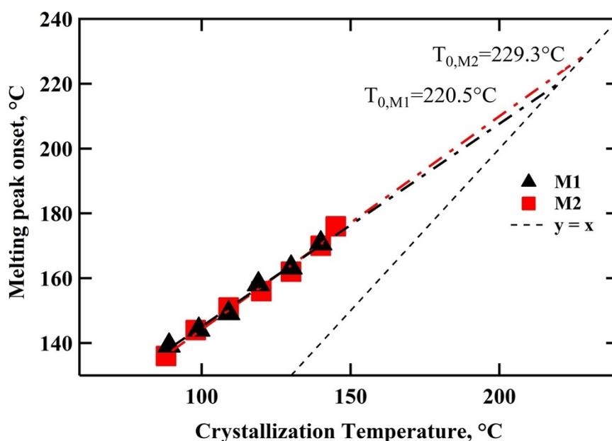
Fig. S1. Dependence of the melting peak onset on the crystallization temperature ( $T_m$  vs.  $T_c$ ). The thermodynamic melting points of M1 and M2 ( $T_{0,M1}$  and  $T_{0,M2}$ , respectively) are determined as the intersection points of the  $T_m$  vs.  $T_c$  curves with the  $T_m = T_c$  line.
