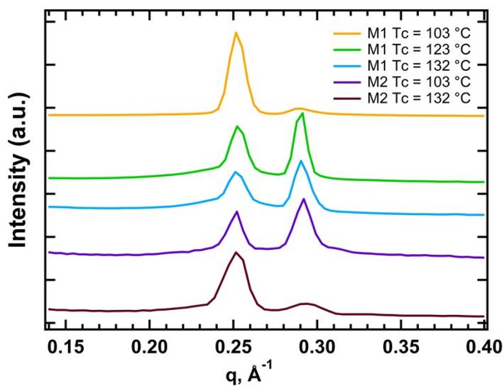
Fig. S3. Room-temperature 1D-reduced X-ray scattering profiles of sample M1, isothermally crystallized at the indicated temperatures.
