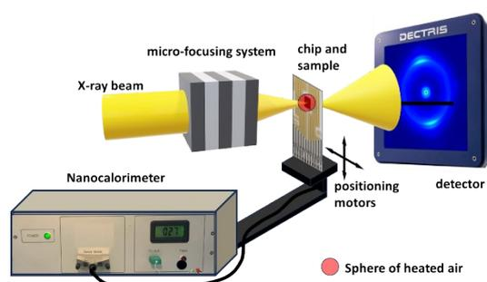
Scheme S1. Combination of nanofocus X-ray diffraction and fast scanning chip calorimetry experimental setup.
