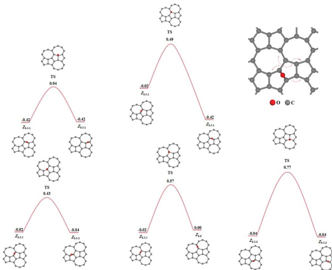
**Fig. S2** Extra oxygen migration pathways on the OPG-Z. The energy value of  $Z_{8.8}$  is shifted to 0 eV. The non-equivalent carbon sites are labeled by the same notations used in Fig. 2. The direction of the arrow indicates the possible pathways of the oxygen migration.
