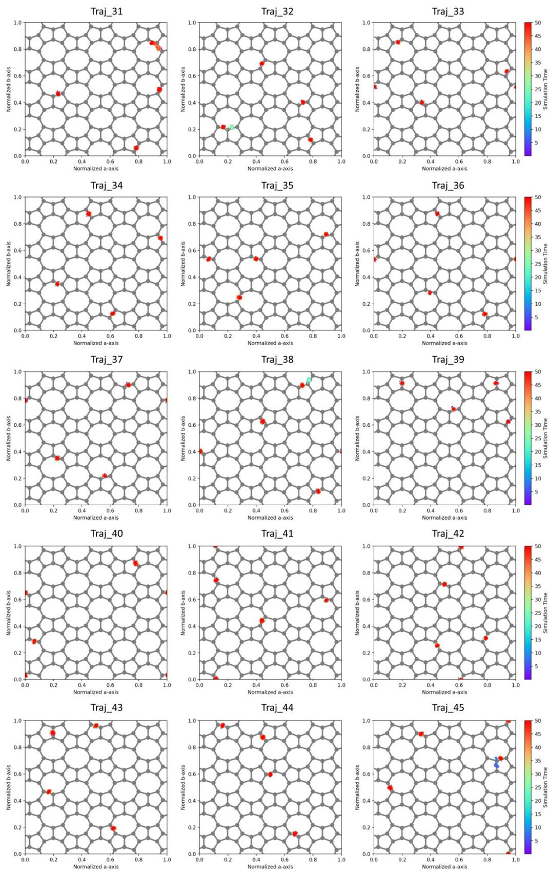
**Fig. S3** MLMD simulations trajectories of oxygen migration on OPG-*L* and OPG-*Z*, respectively. The colored dots denote the positions of 4 oxygen atoms, and the colors denote the simulation time. The static OPG monolayer is used as the background for clarity.
