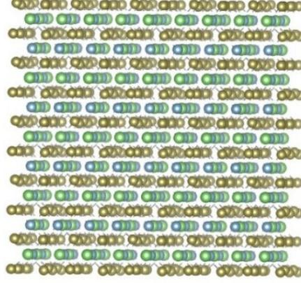
**Fig. S1** The  $4 \times 4 \times 2$  supercell (containing 512 atoms) of  $\alpha$ -LiAlTe<sub>2</sub>, which crystallizes as the tetragonal structure with space group  $I42d$ .
