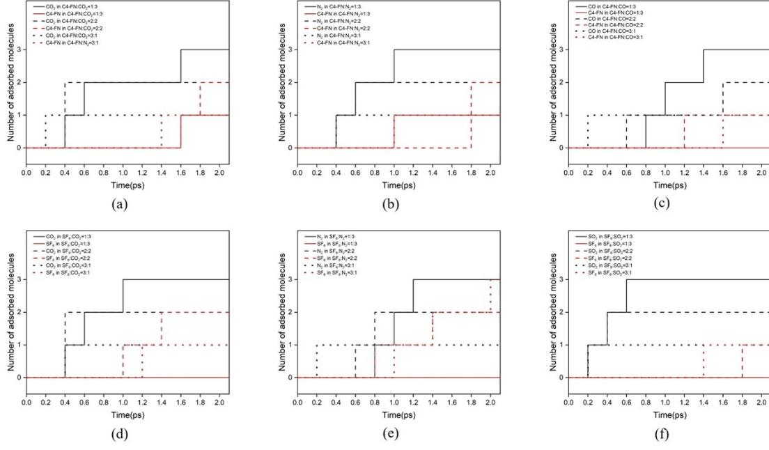
Fig. S5 Tracking the adsorbed molecules in FPMD simulations at 300 K for insulating gases: (a):  $CO_2/C_4F_7N$ ; (b):  $N_2/C_4F_7N$ ; (c):  $CO/C_4F_7N$ ; (d):  $CO_2/SF_6$ ; (e):  $N_2/SF_6$ ; (f):  $SO_2/SF_6$ .
