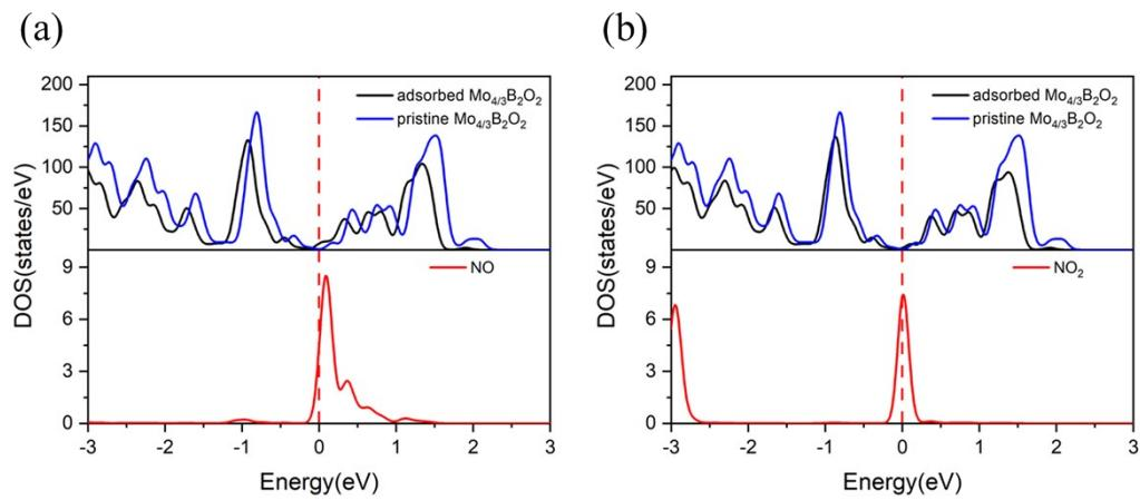
Fig. S3 TDOS of the  $\text{Mo}_{4/3}\text{B}_2\text{O}_2$  substrate with and without the gas adsorbates and the gas molecule along: (a): NO; (b):  $\text{NO}_2$ .
