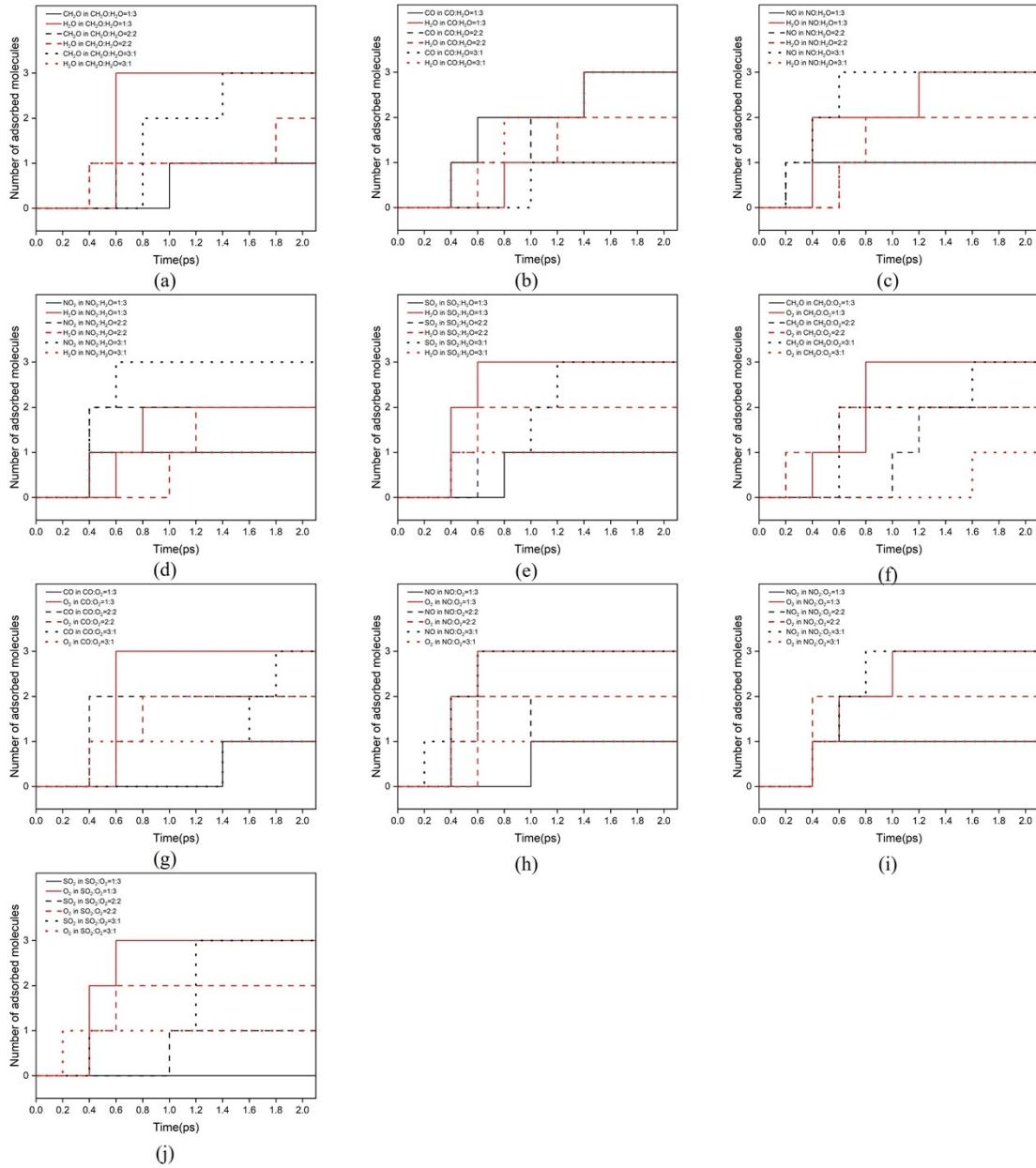
Fig. S7 Tracking the adsorbed molecules for pollutant gases from FPMD simulations at 300 K: (a): CH<sub>2</sub>O/H<sub>2</sub>O; (b): CO/H<sub>2</sub>O; (c): NO/H<sub>2</sub>O; (d): NO<sub>2</sub>/H<sub>2</sub>O; (e): SO<sub>2</sub>/H<sub>2</sub>O; (f): CH<sub>2</sub>O/O<sub>2</sub>; (g): CO/O<sub>2</sub>; (h): NO/O<sub>2</sub>; (i): NO<sub>2</sub>/O<sub>2</sub>; (j): SO<sub>2</sub>/O<sub>2</sub>.
