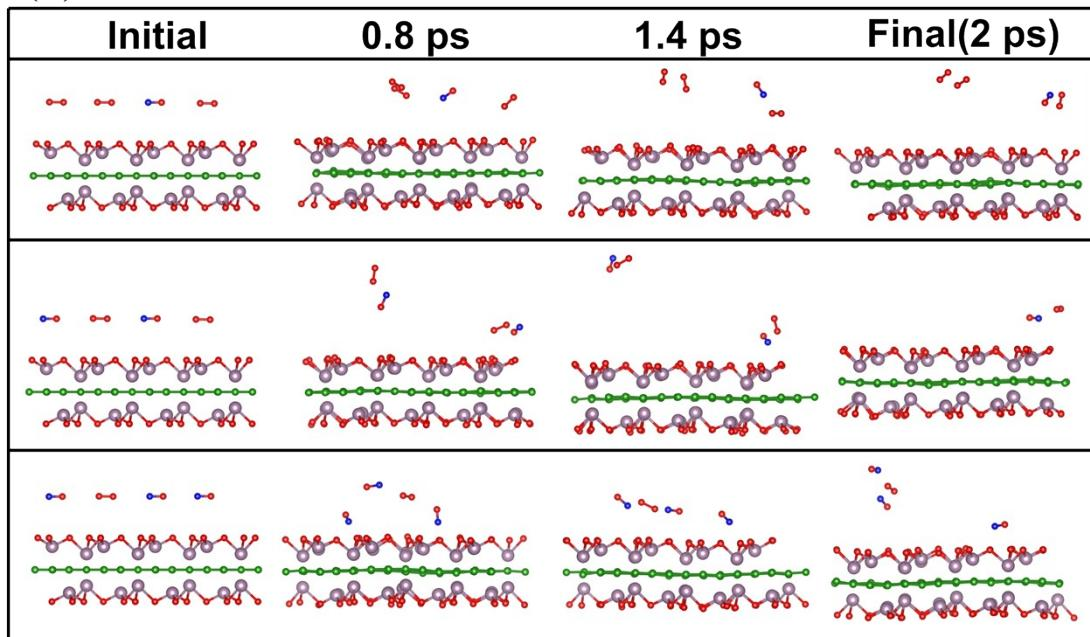
Fig. S8 Molecular dynamics sampling of NO adsorption configurations on  $\text{Mo}_{4/3}\text{B}_2\text{O}_2$  in gas mixtures with different molecular ratios (1:3, 1:1 and 3:1) at 300 K and different times: (a):NO- $\text{H}_2\text{O}$ ; (b): NO- $\text{O}_2$ .
