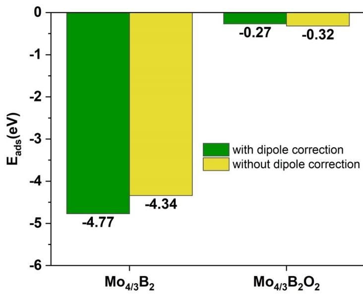
Fig. S1 Adsorption energies of NO on  $\text{Mo}_{4/3}\text{B}_2$  and  $\text{Mo}_{4/3}\text{B}_2\text{O}_2$  with and without dipole correction.
