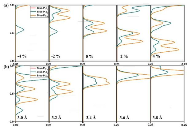
**Figure S6** The contributions of each  $p$  orbital sub-orbital to the CBM of the Blue-P monolayer in Blue-P/SbN vdWHs under (a) Different biaxial strains, and (b) Different interlayer distances.
