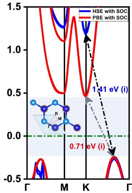
**Figure S1** The band structures of the most stable configuration (hcp-top) of Blue-P/SbN vdWHs were calculated using both PBE+SOC and HSE06+SOC methods.
