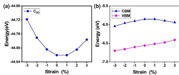
**Figure S4** (a) Total energy variation curves of heterostructure under different strains, (b) Change curve of CBM and VBM under different strains.
