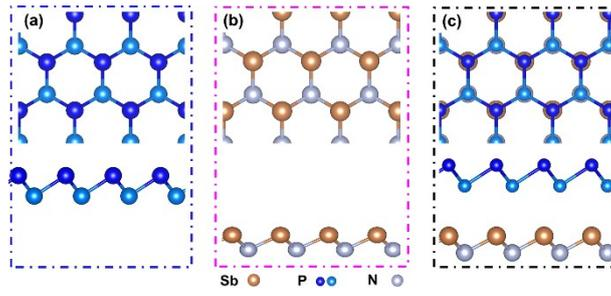
**Figure S2** (a)-(c) The geometric structures of Blue-P monolayer, SbN monolayer, and the most stable configurations of Blue-P/SbN vdWHs, respectively.
