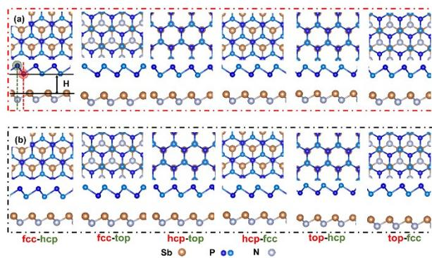
**Figure S3** Top and side views of six high symmetry structures of Blue-P/SbN vdWHs. (a) Initial structures and (b) optimized structures, respectively. The yellow, dark (light) blue, and gray balls represent Sb, P and N atoms, respectively.
