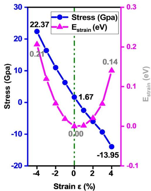
**Figure S5** Strain energy ( $E_{\text{strain}}$ ) and stress-strain curves of Blue-P/SbN vdWHs were calculated. The blue line represents the change of stress-strain, the pink line represents the change of strain energy.
