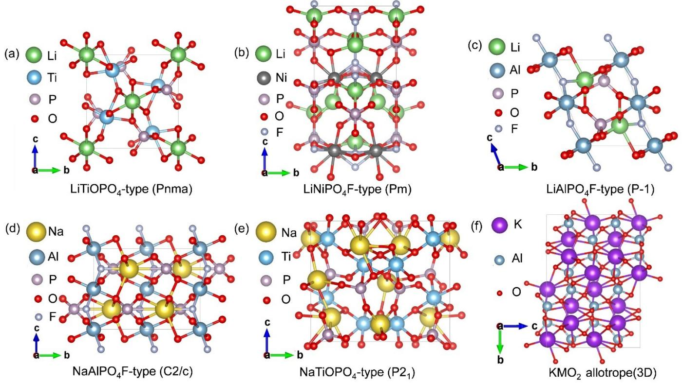
**Figure S1.** The orthogonal KTiOPO<sub>4</sub> (Pna21) structure of the corresponding Li and Na analogues forms a total of five different structures, specifically including (a) LiTiOPO<sub>4</sub>-type (Pnma), (b) LiNiPO<sub>4</sub>F-type (Pm), (c) LiAlPO<sub>4</sub>F-type (P-1), (d) NaAlPO<sub>4</sub>F-type (C2/c), and (e) NaTiOPO<sub>4</sub>-type (P2<sub>1</sub>). (f) The only isomer with 3D structure of the layered KMO<sub>2</sub> solid electrolyte candidate material.
