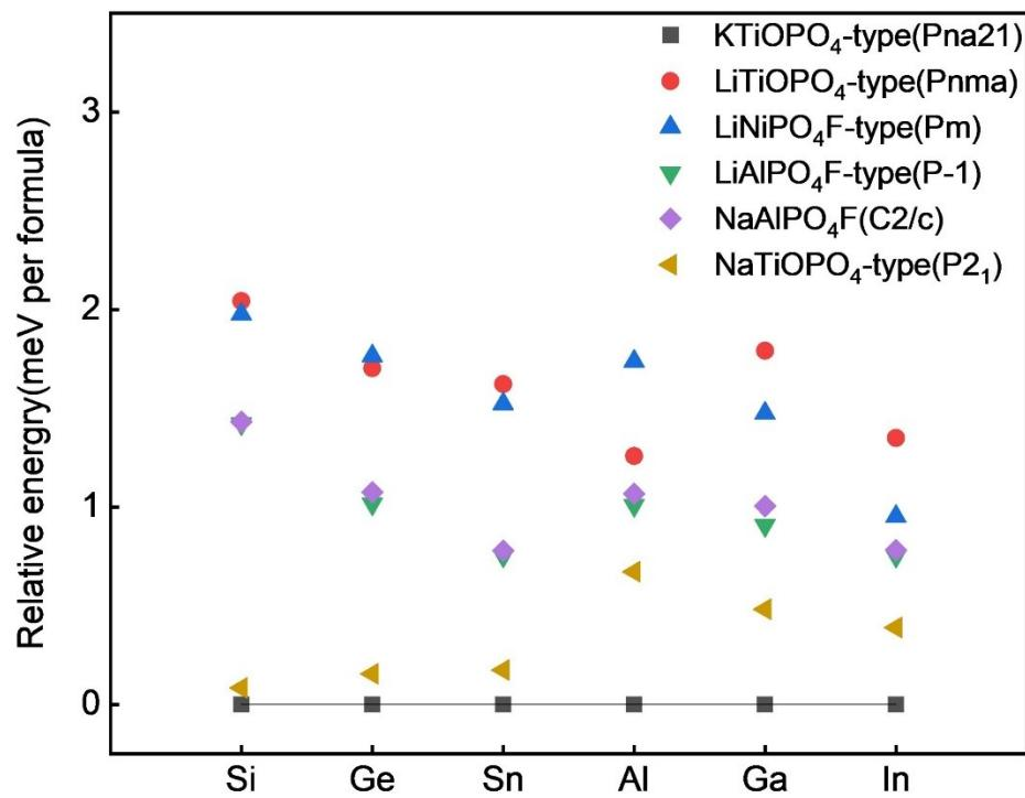
**Figure S2.** The relative energies of the five spatial group isomers of the orthogonal KTiOPO<sub>4</sub>-type(Pna21) structure and its corresponding Li/Na analogues.
