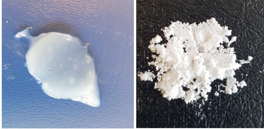
Fig. S3 Synthetic C-S-H produced in the segmented flow tubular reactor (SFTR) after filtration (left) and freeze-drying (right).
