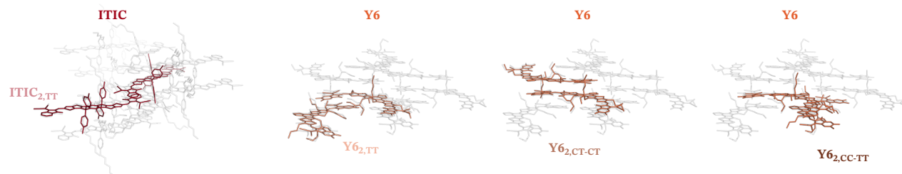
Fig. S11 Comparison of crystal structures for ITIC 15 and Y6 17 with the different geometry-optimised dimers ITIC 2,TT , Y6 2,TT , Y6 2,CT-CT , and Y6 2,CC-TT . The geometries were optimised at the BP86/def2-SVP level in ORCA.
