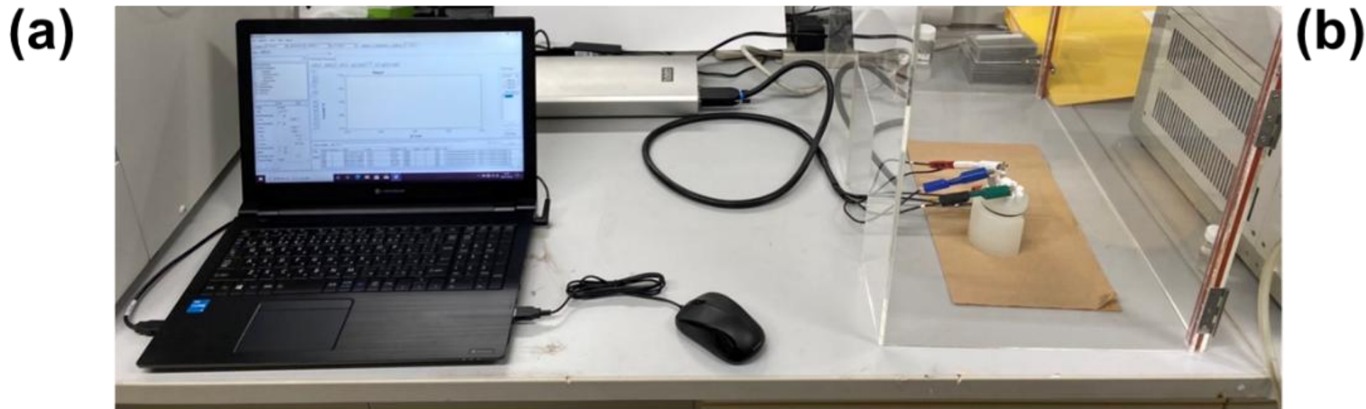
Figure S1. (a) Overview of the electrochemical measurement instrument consisted of a triode cell, a potentiostat (Vertex 1A), and an analysis PC (IviumSoft). (b) Triode glass cell (HX-111), containing a working electrode of glassy carbon (HX-W8, center), a counter electrode with platinum (HX-C13, left), and the reference electrode of Ag/AgCl (HX-R14, right).
