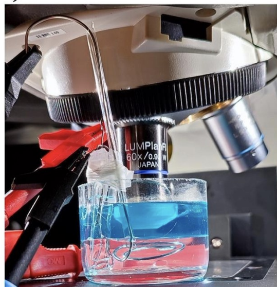
Figure S2: (A) Photographs of the electrochemical cell used for Raman spectroelectrochemical experiments. (B) 4-electrode spectroelectrochemical cell with an immersion objective used for the SERS experiments on electrogenerated AuNP films. The aqueous solution contained methylene blue.
