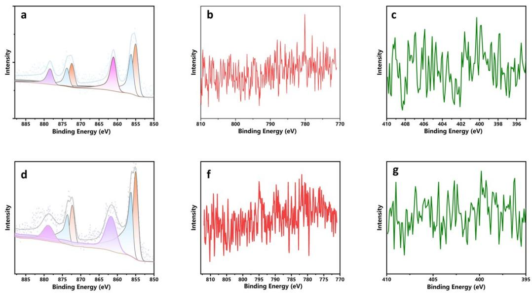
**FigS6 XPS test results: 1000 rounds of CV test results a)Ni, b)Co, c)N,**
