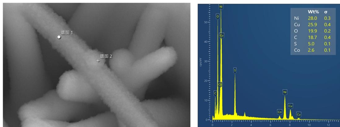
FigS3 SEM-EDS point scanning results and the elemental composition ratios
