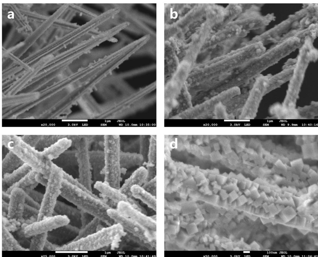
FigS1 a) PBAs loaded on nanowires synthesized in 1M NaOH b) PBAs generated
