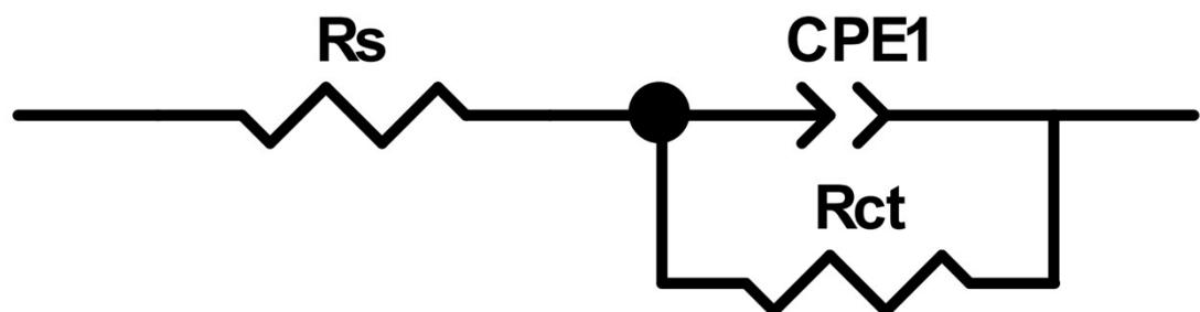
**FigS5** EIS equivalent circuit
