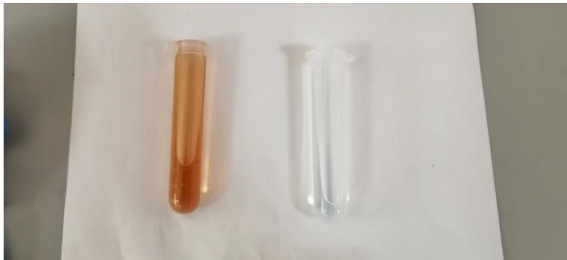
**Fig S14** After long-term standing (>2 days) following the electrocatalytic reaction, whether further electrocatalytic reactions occur can be assessed by comparing the states of the pure Ni foam (left) and the target catalyst (right), both of which have completed the full electrolysis process
