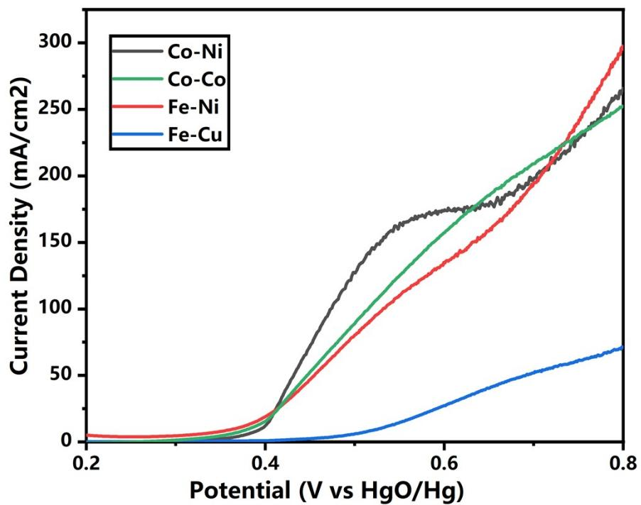
**FigS9 Comparison of Linear Sweep Voltammetry (LSV) results under different elemental combinations**
