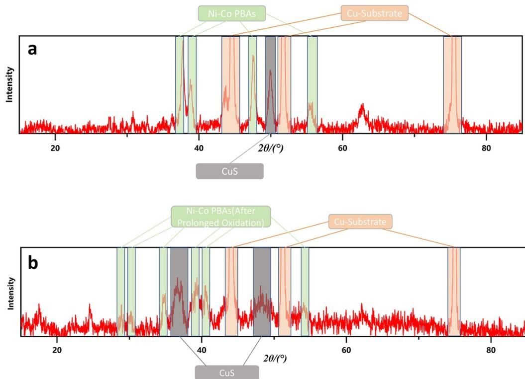
**FigS7 XRD patterns: a) prepared sample b) after prolonged electrocatalytic oxidation**
