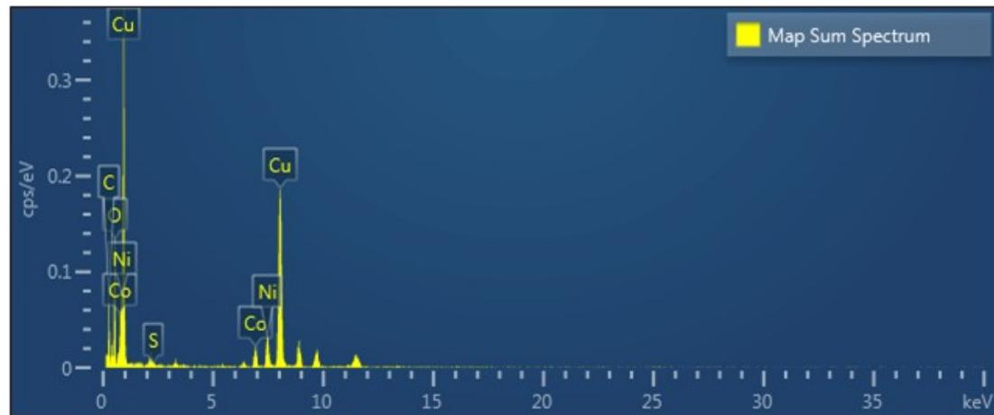
FigS2 TEM-EDX mapping test results and elemental ratios
