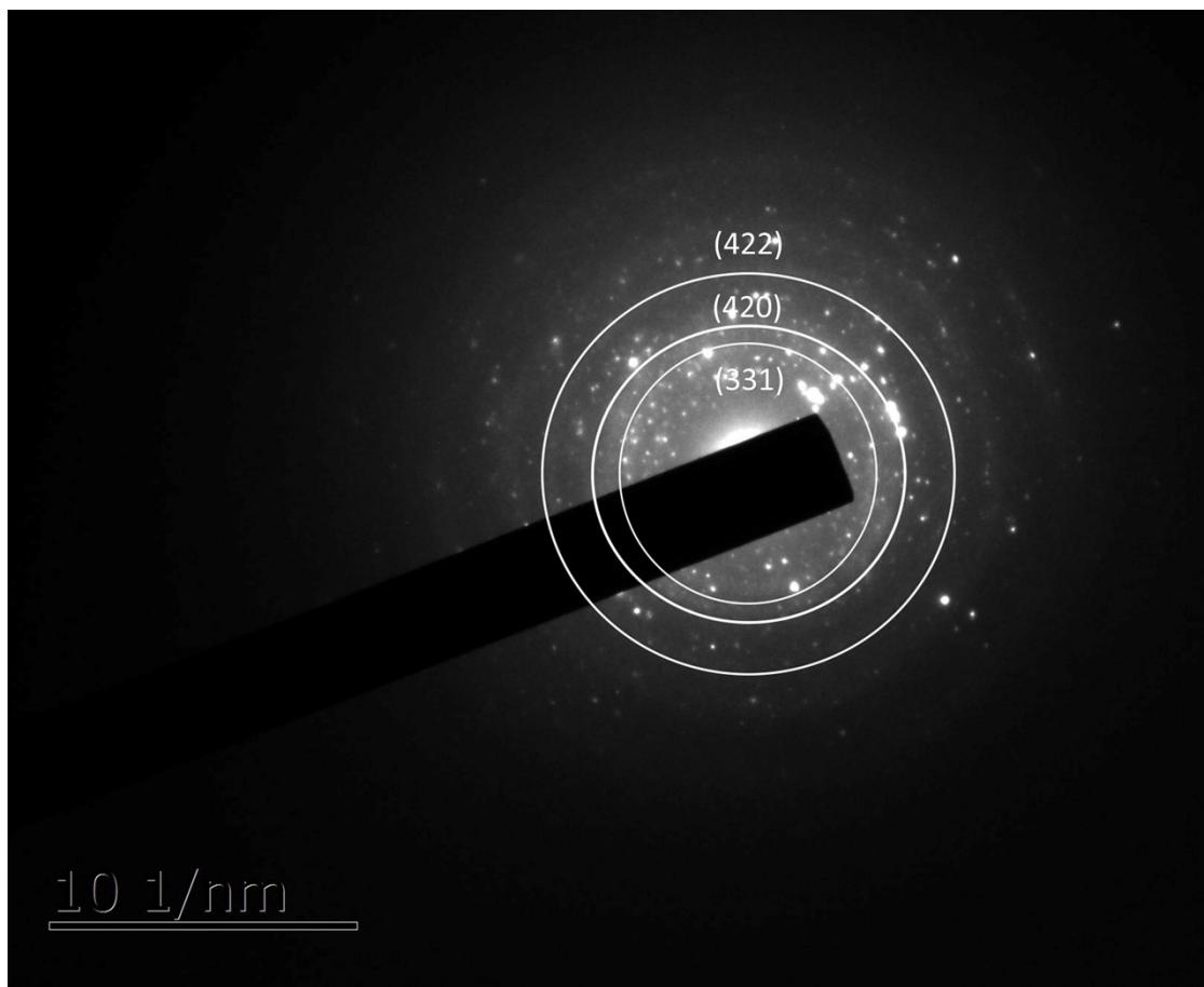
**FigS4** SAED test results and markings
