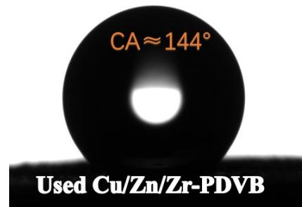
Figure S7. The water contact angle of used Cu/Zn/Zr-PDVB catalyst.
