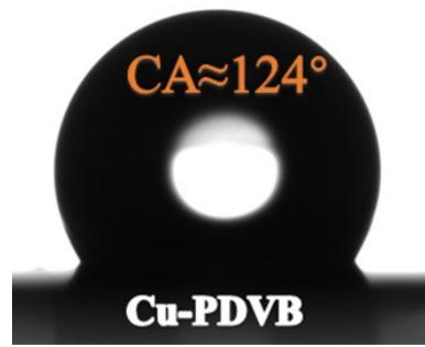
Figure S1. The water contact angle of Cu-PDVB catalyst.
