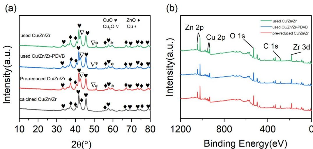
Figure S5. XRD (a) and XPS (b) spectrogram of Cu/Zn/Zr Catalyst.
