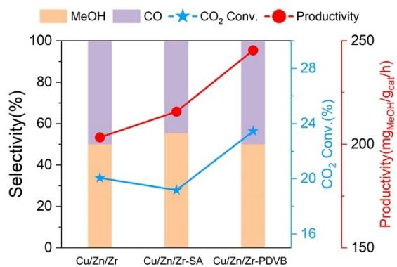
Figure S3. Catalytic performance of stearic acid modified Cu/Zn/Zr Catalyst.
