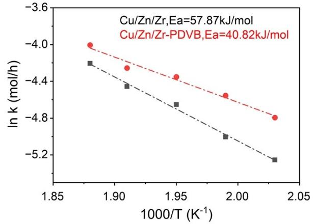
Figure S9. The Arrhenius plots for  $\text{CO}_2$  hydrogenation were conducted over  $\text{Cu}/\text{Zn}/\text{Zr}$  and  $\text{Cu}/\text{Zn}/\text{Zr-PDVB}$  catalysts.
