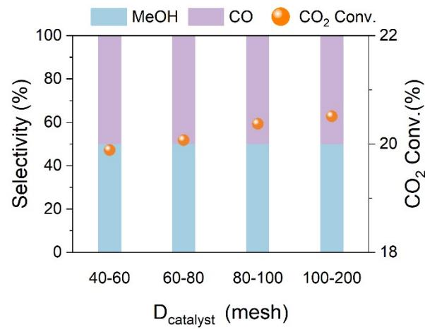
Figure S4. Catalytic performance of Cu/Zn/Zr Catalysts with different particle sizes.
