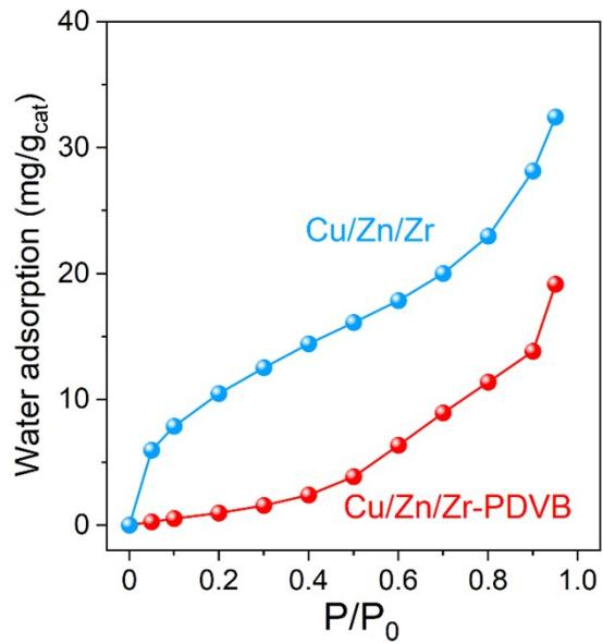
Figure S12. Water vapor adsorption test of Cu/Zn/Zr and Cu/Zn/Zr-PDVB catalysts.
