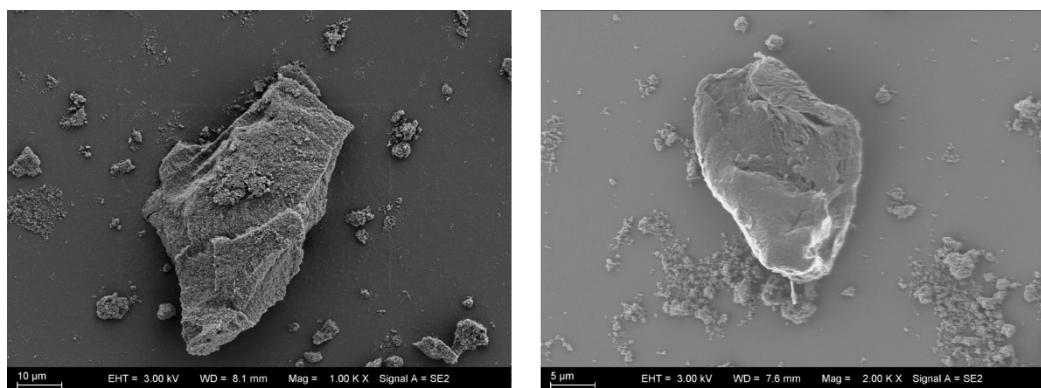
Figure S8. SEM images of PDVB before (left) and after (right) reaction.
