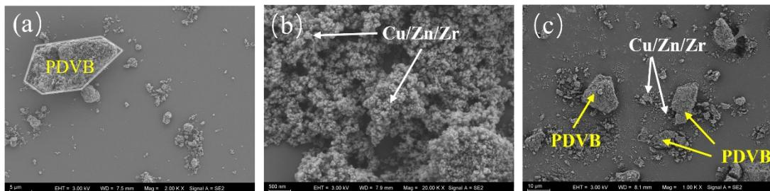
Figure S11. SEM images of PDVB (a),  $\text{Cu}/\text{Zn}/\text{Zr}$  (b), and  $\text{Cu}/\text{Zn}/\text{Zr-PDVB}$  (c).
