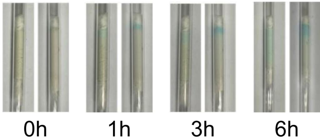
Figure S13. Photos of anhydrous CuSO<sub>4</sub> mixed with PDVB (left) and anhydrous CuSO<sub>4</sub> mixed with quartz powder (right) with H<sub>2</sub>O/N<sub>2</sub> (30 mL/min) flow at room temperature for different periods.
