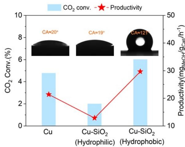
Figure S2. Catalytic performance of Cu-SiO<sub>2</sub> Catalyst with different wettability.
