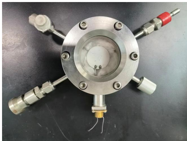
Fig S9. Photograph of home-made reactor for photothermal and thermal catalytic ammonia synthesis.
