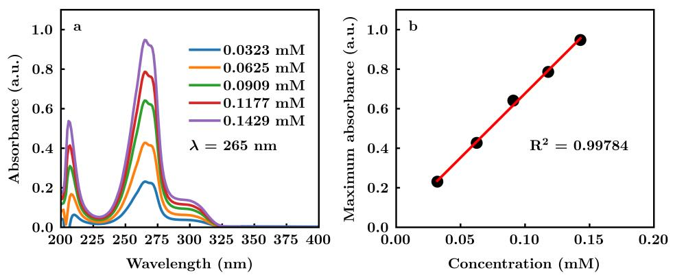
**Fig. S3** (a) UV-Vis spectra of N-[(pyrazin-2-yl)methyl]formamide at various concentrations. (b) Standard calibration curve plotting absorbance at  $\lambda = 265$  nm against concentration for N-[(pyrazin-2-yl)methyl]formamide.
