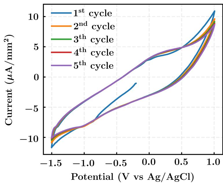
**Fig. S2** Cyclic voltammograms of 1M KCl electrolyte background solution, scanned at a rate of 20 mV/s.
