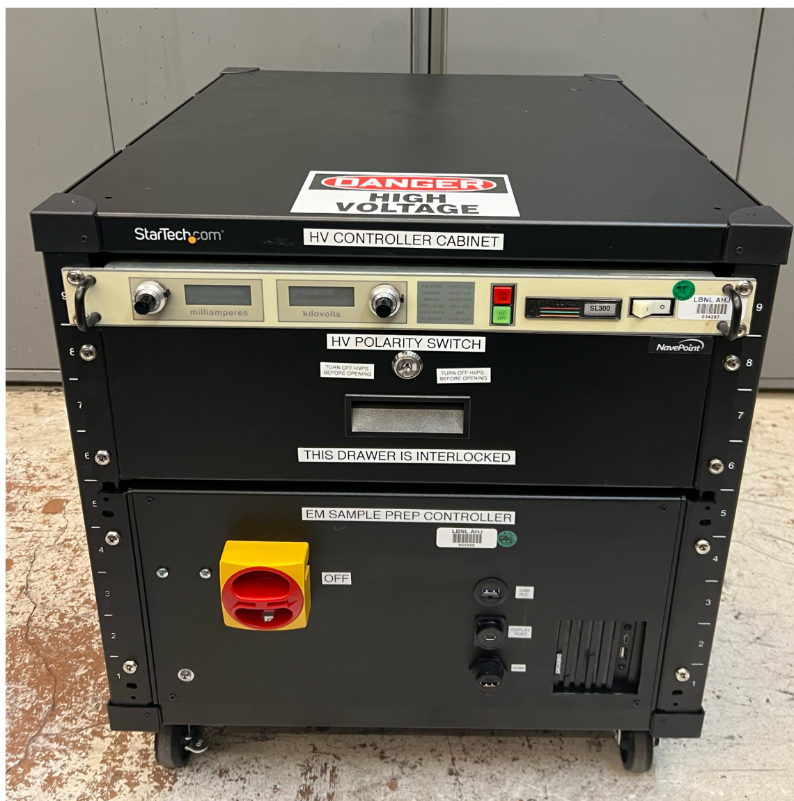
Supplementary Figure S1: Control panel chassis for the EMSBot.
