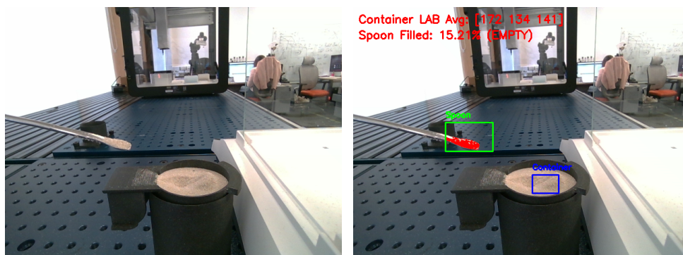
Figure 2: False negative classification of scooped SiO_2 : the scoop was flagged by the vision system as having insufficient material with P_{fill} = 15.21 , below the required threshold t_{empty} = 16 . The measured quantity however was 25.2 mg.
