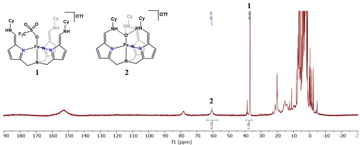
**Figure S1.** A representative  $^1\text{H}$  NMR spectrum from the generation of the calibration curve (test 2, entry 10) (500 MHz,  $\text{CD}_3\text{CN}$ ).
