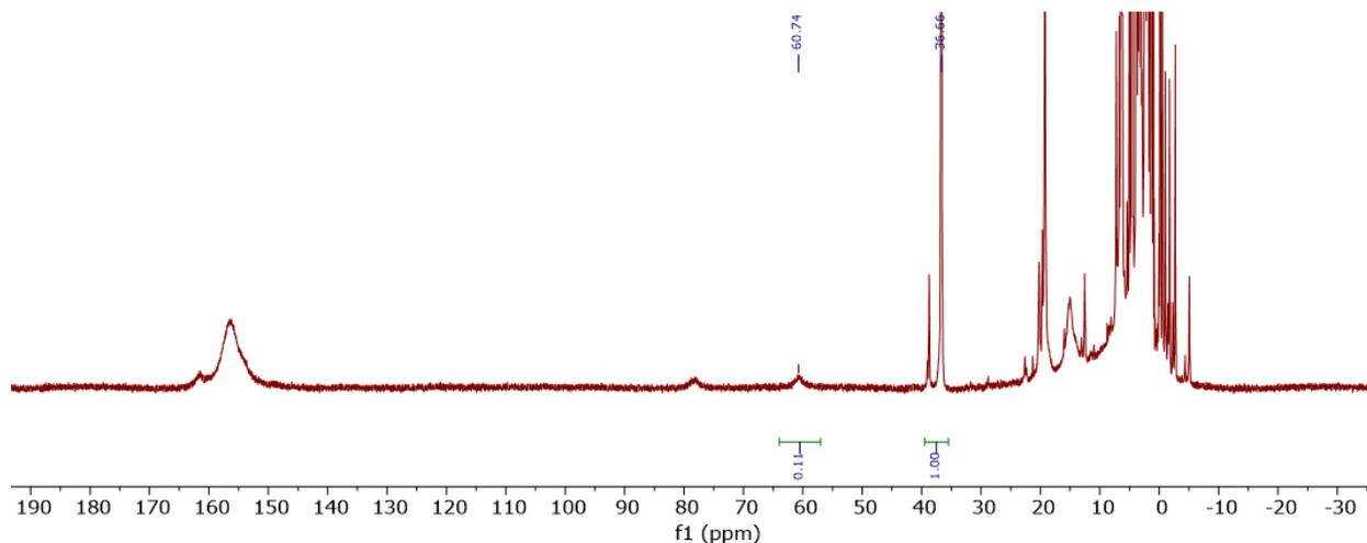
**Figure S5.** A representative  $^1\text{H}$  NMR spectrum of the reduction of  $[\text{TBA}]_2\text{Cr}_2\text{O}_7$  by **1** (trial 2, aliquot A) (500 MHz,  $\text{CD}_3\text{CN}$ ).
