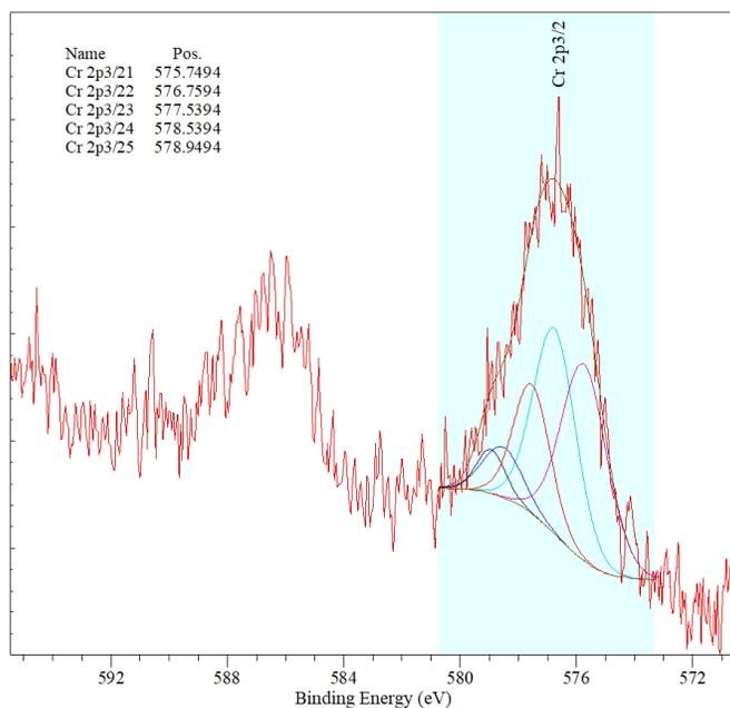
**Figure S6.** XPS analysis of the precipitated material from the large scale reduction of  $[\text{TBA}]_2\text{Cr}_2\text{O}_7$ .
