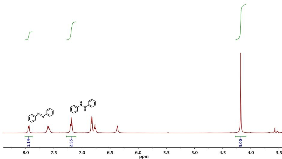
**Figure S3.**  $^1\text{H}$  NMR spectrum of the quantification of chromate reduction using 1,2-diphenylhydrazine, demonstrating the formation of 2.47 equiv of **2** (500 MHz,  $\text{CD}_3\text{CN}$ ).
