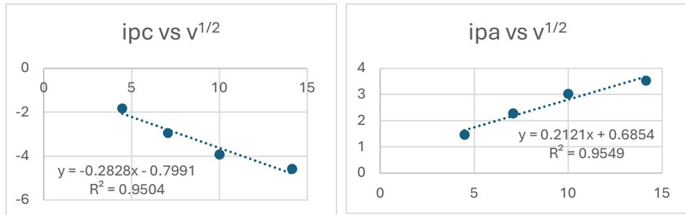
Figure S36: Plots of  $i_{pa}$  and  $i_{pc}$  vs  $v^{1/2}$  for the process at  $E_{1/2} = -1.67$  V in (2-Co)
