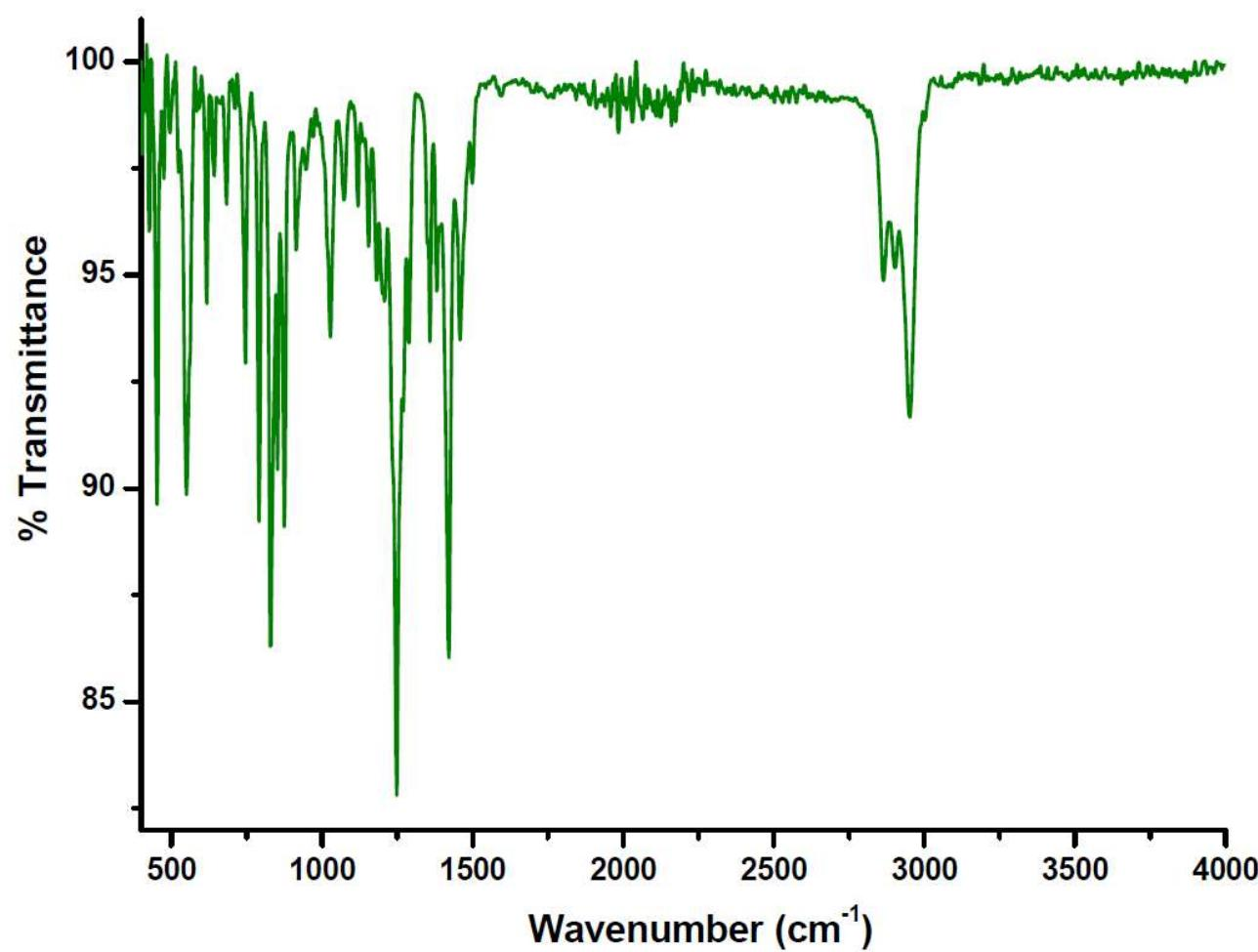
Figure S20a: The solid state IR spectrum of (2-Co.THF).
