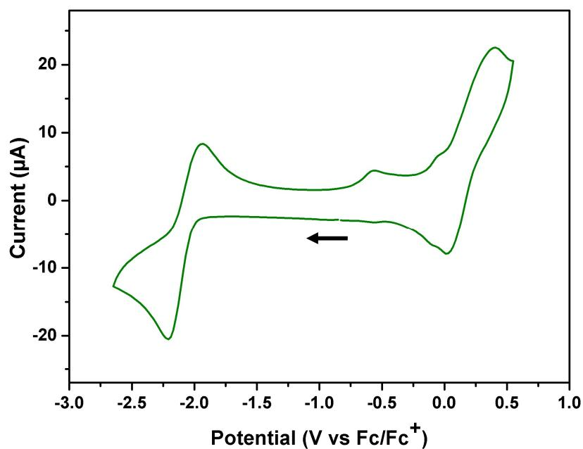
Figure S30a: The Cyclic voltammogram (one scan) of (**2-Fe**) measured cathodically with a scan rate of 200 mV/s; 5 mg of (**2-Fe**) (2.7 mM) and 121 mg of TBAPF<sub>6</sub> (*ca* 0.1M) in 3 ml of 1,2-difluorobenzene.
