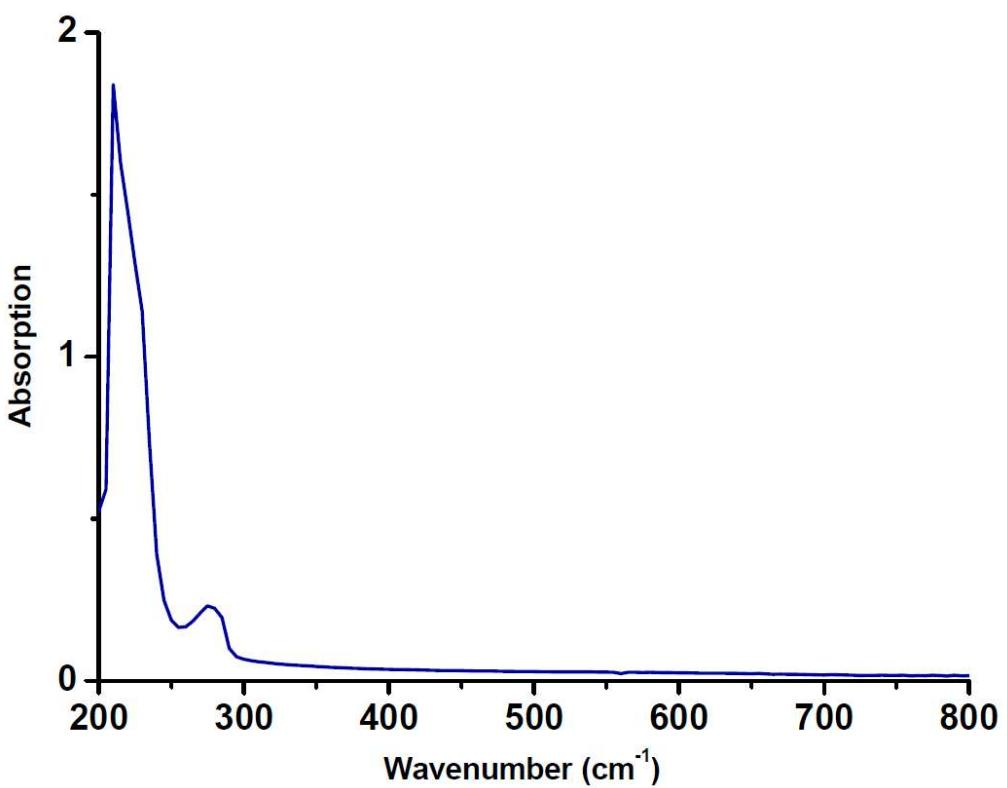
Figure S25: UV-Vis spectrum of (2-Co.THF) measured as a 45  $\mu\text{M}$  THF solution;  $\lambda = 275 \text{ nm}$ ,  $\epsilon = 5133 \text{ cm}^{-1}\text{M}^{-1}$ .
