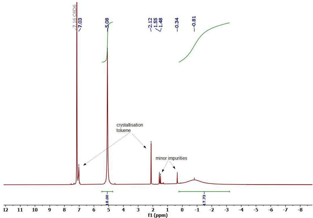
Figure S6: The  ${}^1\text{H}$  NMR spectrum ( $\delta(\text{C}_6\text{D}_6)$ ) of **(2-Fe)** in the region between -8 to 12 ppm.
