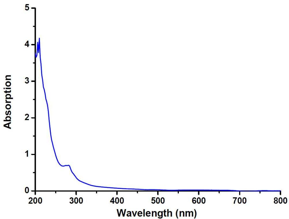
Figure S22: UV-Vis spectrum of (**2-Fe**) measured as a 80 $\mu$ M n-hexane solution;  $\lambda = 282$  nm,  $\epsilon = 8937.5 \text{ cm}^{-1}\text{M}^{-1}$
