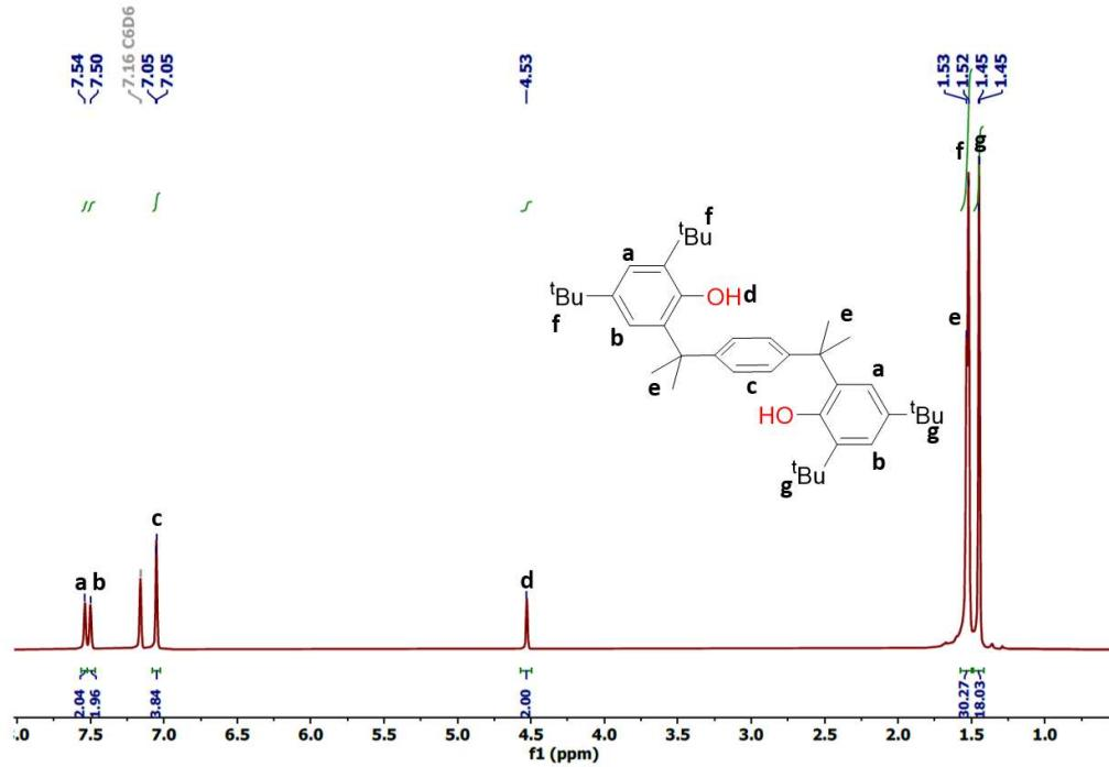
Figure S1: The  $^1\text{H}$  NMR spectrum of  $\text{LH}_2$  measured in  $\text{C}_6\text{D}_6$ .
