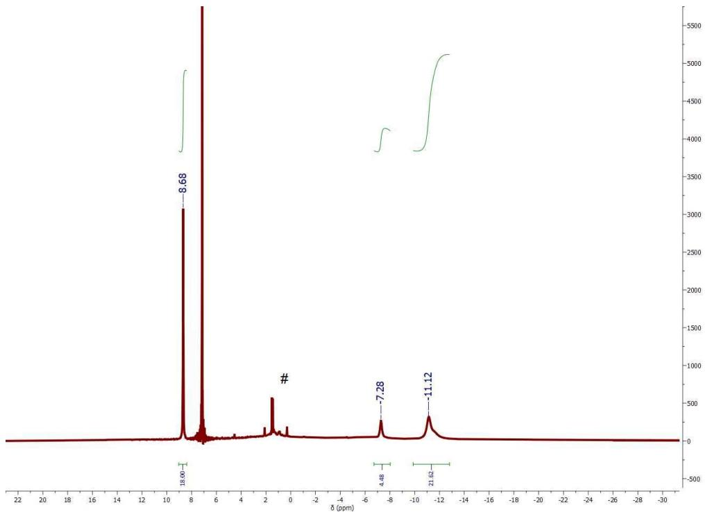
Figure S14: The  $^1\text{H}$  NMR ( $\delta(\text{C}_6\text{D}_6)$ ) of (2-Co.THF) in the region between -30 to 22 ppm; # denotes minor impurities.
