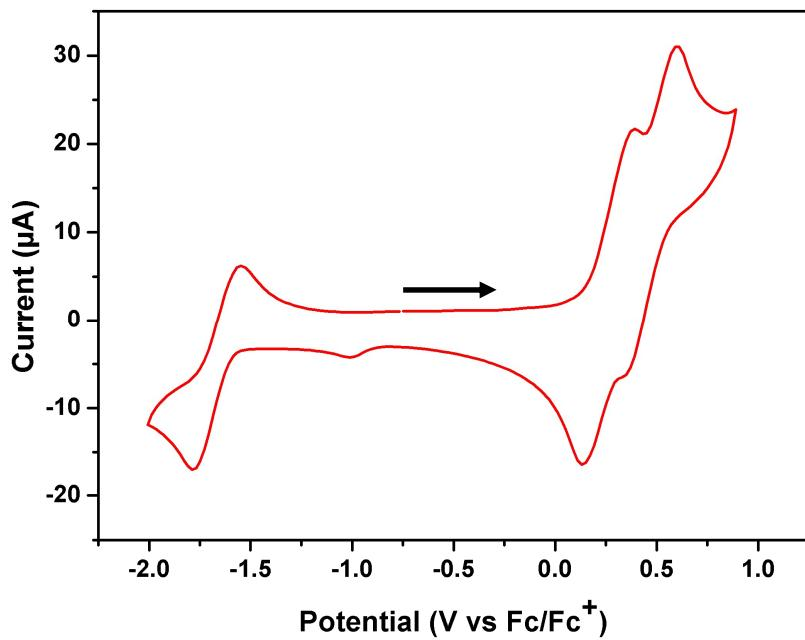
Figure 31b: The CV (1 scan) of **(2-Co)** measured anodically with a scan rate of 200 mV/s; Conditions: 5 mg of **(2-Co)** (1.5 mM) and 121 mg of TBAPF<sub>6</sub> (0.06 M) in 5 ml of 1,2-difluorobenzene.
