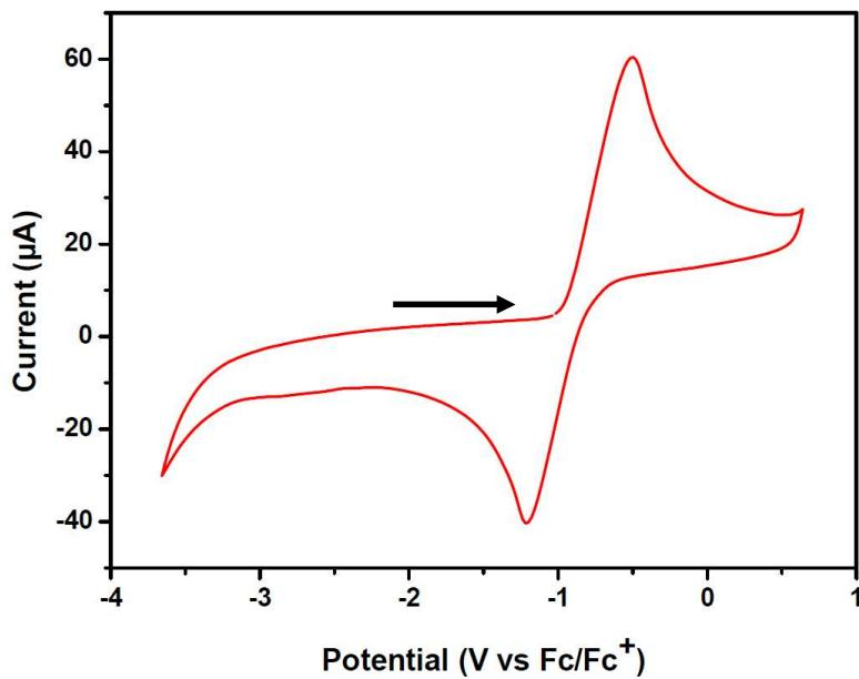
Figure S34: The Cyclic voltammogram (2<sup>nd</sup> scan) of (**2-K<sub>2</sub>**) salt measured anodically with a scan rate of 200 mV/s. Conditions: 5 mg of (**2-K<sub>2</sub>**) (ca 7.7 mM) and 193 mg of TBAPF<sub>6</sub> (0.17 M) in 3 ml of THF.
