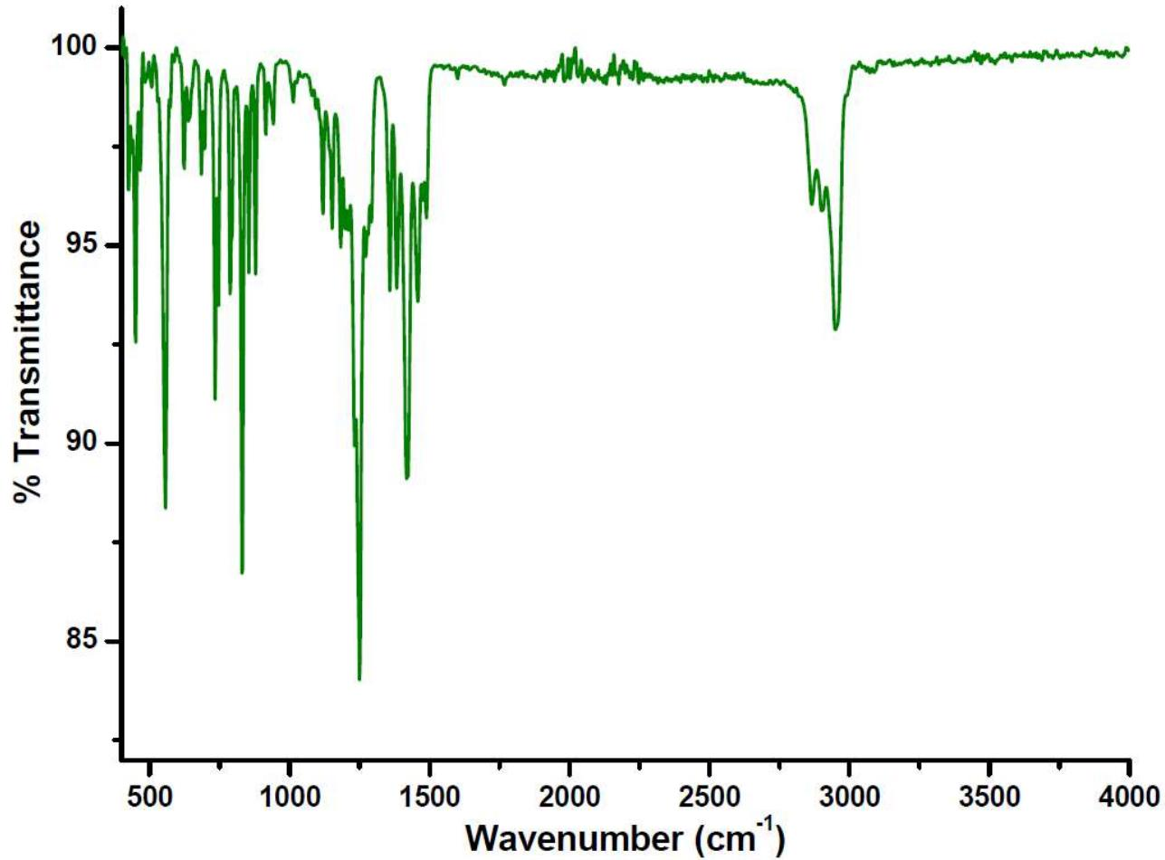
Figure S18a: The solid state IR spectrum of (2-Co).
