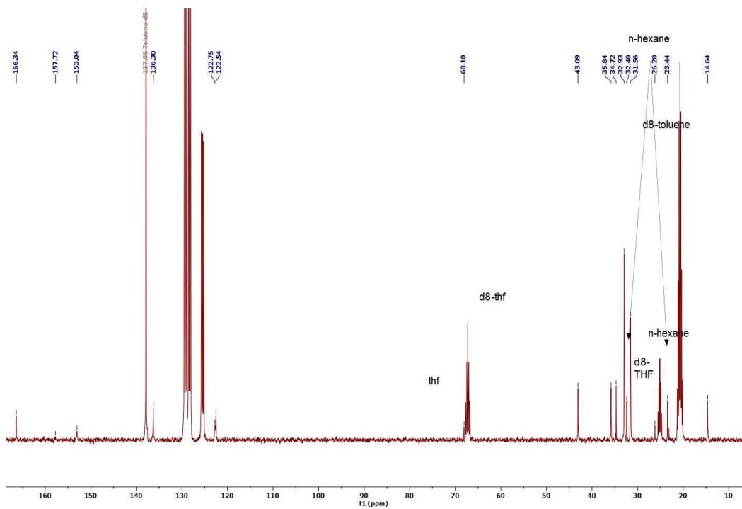
Figure S4: The  $^{13}\text{C}\{^1\text{H}\}$  NMR spectrum of (**2-K<sub>2</sub>**) measured in  $\text{d}^8\text{-toluene}$  with a few drops of  $\text{d}^8\text{-THF}$ .
