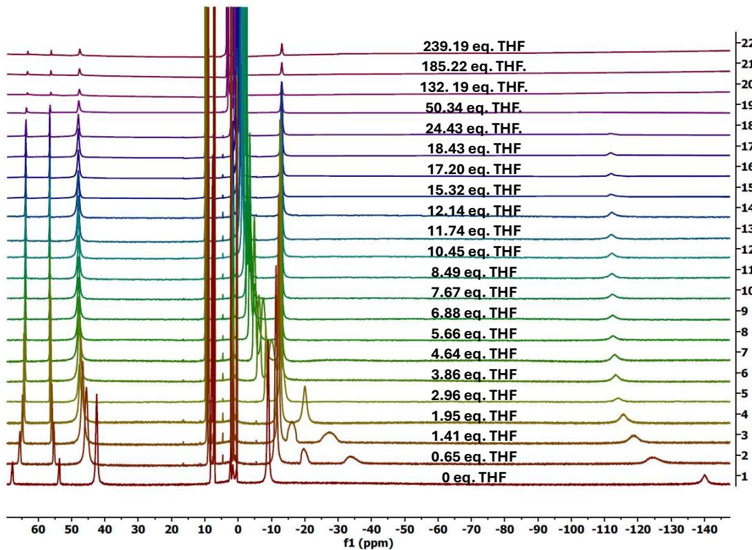
Figure S28: NMR titration experiment on the **(2-Co)** complex measured at 16°C.
