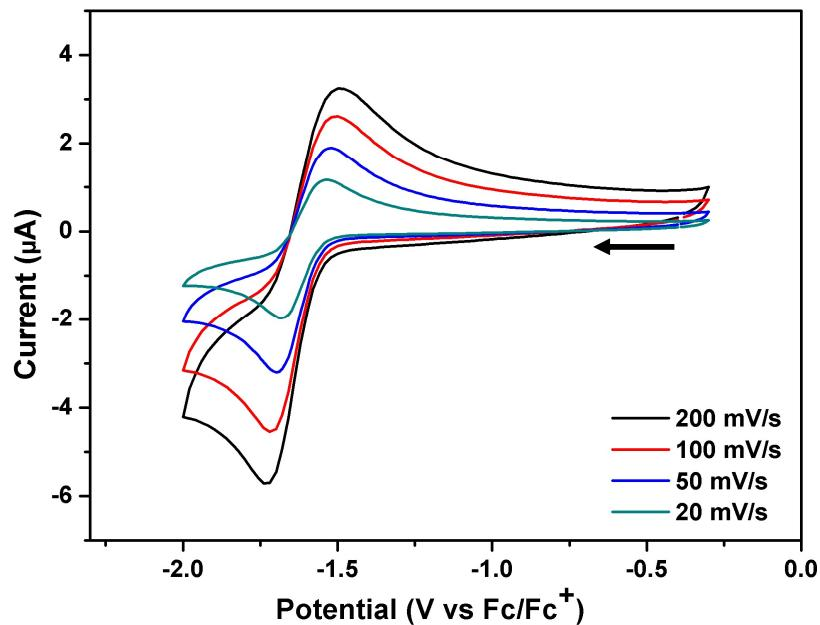
Figure 31c: Overlayed CV's (2<sup>nd</sup> scan) with different scan rates at  $E_{1/2} = -1.67$  V vs  $\text{Fc}^+/\text{Fc}$ . Data have been collected both anodically and cathodically with no effect on the position of the peaks, their separation or current responses. The slight decrease
