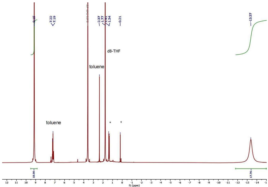
Figure S15: The  $^1\text{H}$  NMR spectrum ( $\delta(\text{d}^8\text{-THF})$ ) of (2-Co.THF) in the region between -15 to 12 ppm; \* denotes minor impurities.
