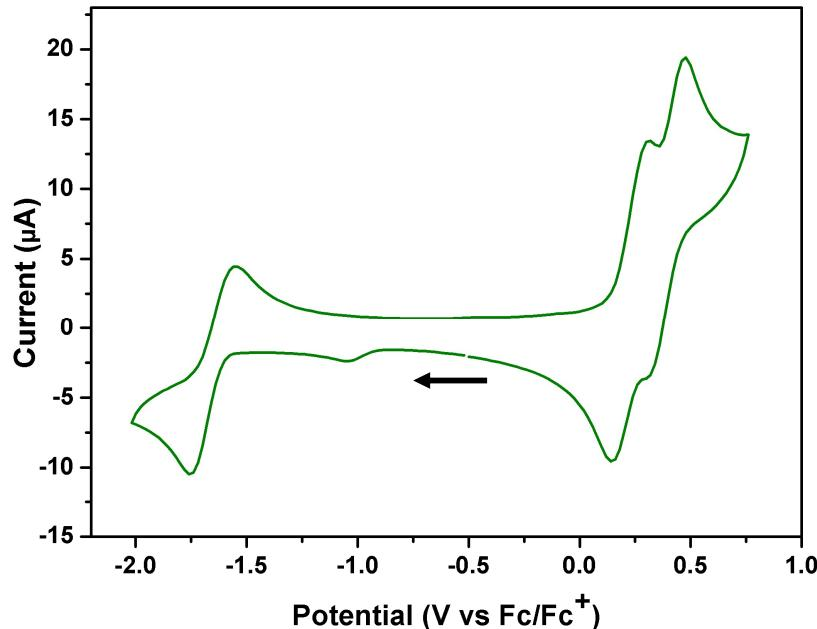
Figure S31a: The CV (one scan) of (**2-Co**) measured cathodically with a scan rate of 200 mV/s; Conditions: 5 mg of (**2-Co**) (1.5 mM) and 121 mg of TBAPF<sub>6</sub> (0.06 M) in 5 ml of 1,2-difluorobenzene.
