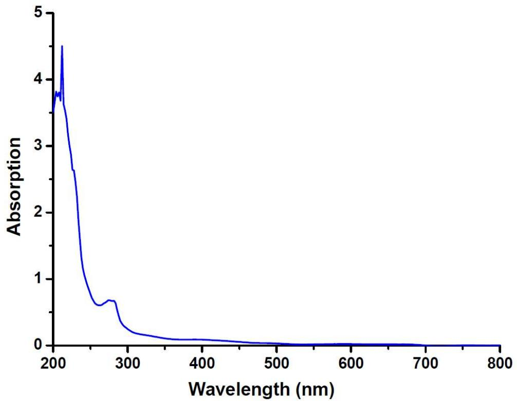
Figure S23: UV-Vis spectrum of (**2-Co**) measured as a 79  $\mu\text{M}$  n-hexane solution;  $\lambda = 282 \text{ nm}$ ,  $\epsilon = 14500 \text{ cm}^{-1}\text{M}^{-1}$ .
