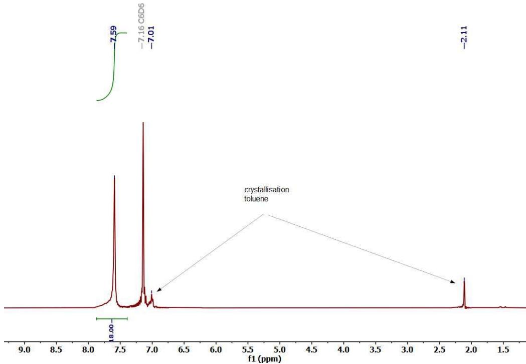
Figure S8: The  $^1\text{H}$  NMR spectrum ( $\delta(\text{C}_6\text{D}_6)$ ) of (2-Co) in the region between 1.5-9.0 ppm
