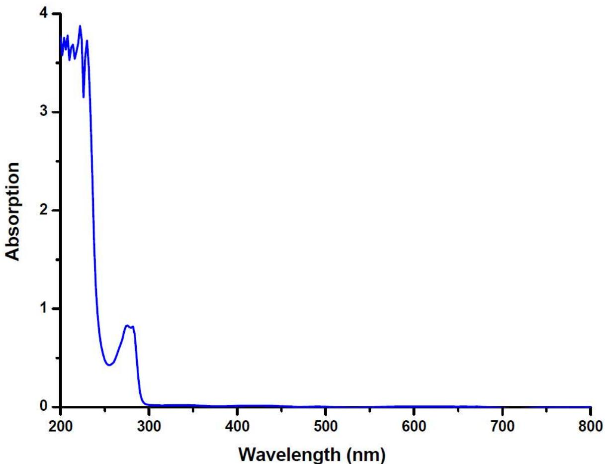
Figure S21: UV-Vis spectrum of LH<sub>2</sub> measured as a 44 μM THF solution; λ=276 nm, ε = 18509.6 cm<sup>-1</sup>M<sup>-1</sup>.
