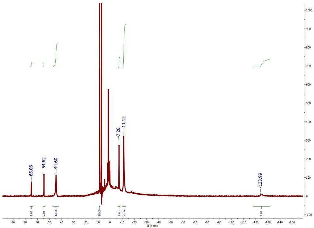
Figure S13: The  $^1\text{H}$  NMR ( $\delta(\text{C}_6\text{D}_6)$ ) of (2-Co.THF) in the region between -160 to 80 ppm
