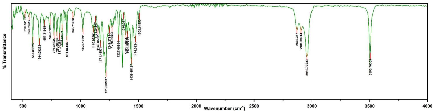
Figure S16b: Peak picked solid state IR spectrum LH<sub>2</sub>.
