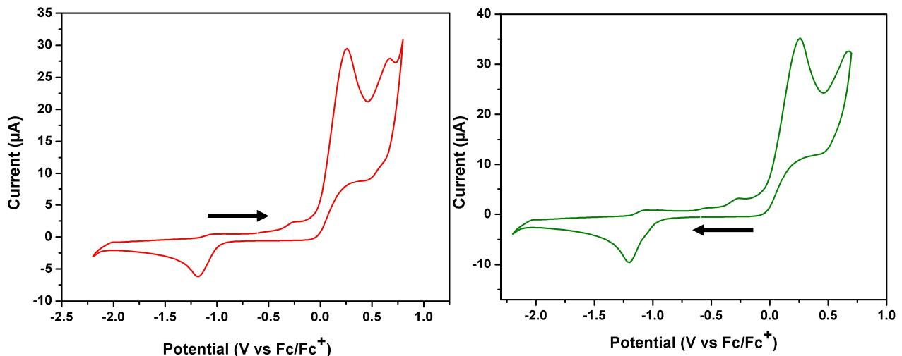
Figure S33: *left*) The Cyclic voltammogram (1st scan) of (2-Co.THF) complex measured anodically with a scan rate of 200 mV/s; *right*) The Cyclic voltammogram (2nd scan) of (2-Co.THF) complex measured cathodically with a scan rate of 200 mV/s;
