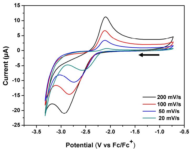
Figure S32b: Expanded picture of the scan rate dependence of the process at *ca* -2.61 V vs  $\text{Fc}^+/\text{Fc}$  observed for complex (2-Fe.THF).
