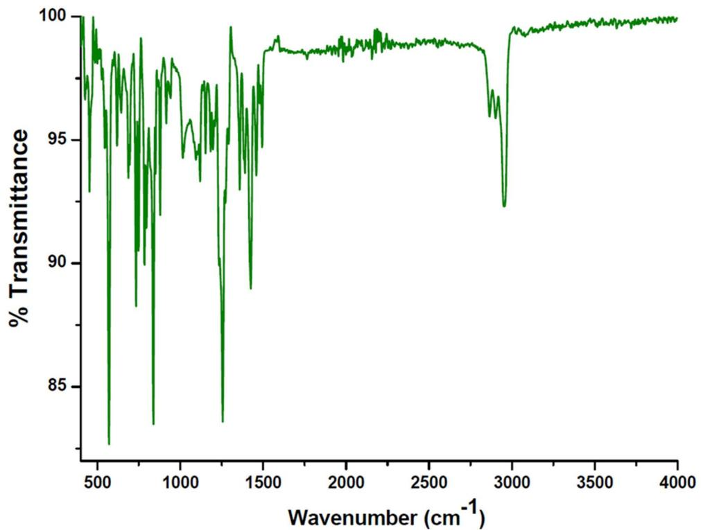
Figure S17a: The solid state IR spectrum of (**2-Fe**).
