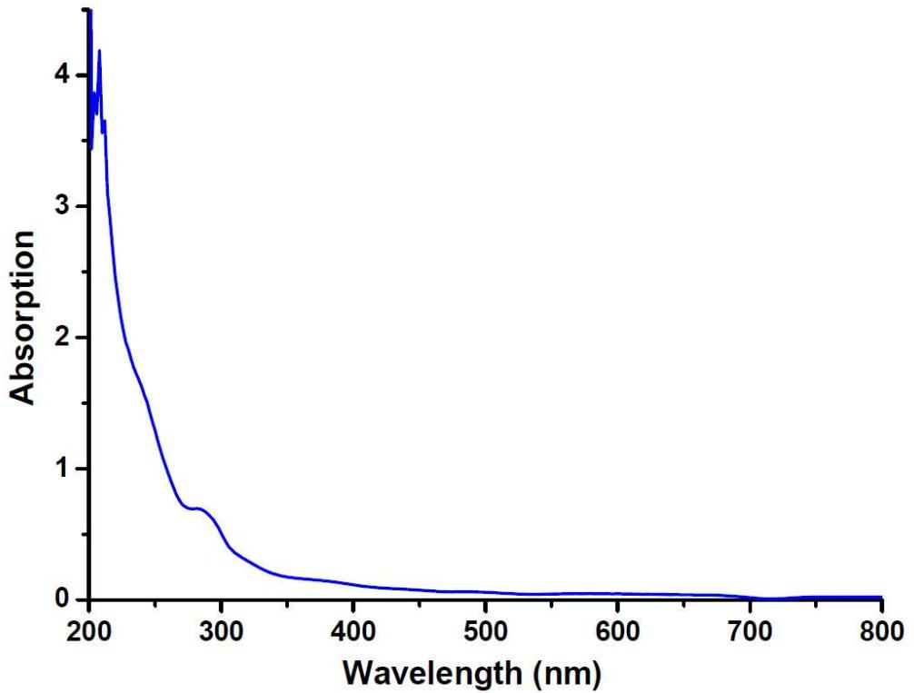
Figure S24: UV-Vis spectrum of (**2**-Fe.THF) measured as a 48  $\mu$ M THF solution;  $\lambda = 282$  nm,  $\epsilon = 14500 \text{ cm}^{-1}\text{M}^{-1}$ .
