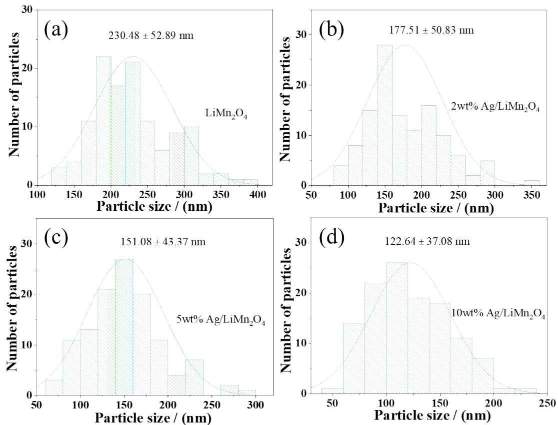
**Fig. S1** (a-d) The particle size distribution of the  $\text{LiMn}_2\text{O}_4$  and Ag-coated  $\text{LiMn}_2\text{O}_4$  samples.
