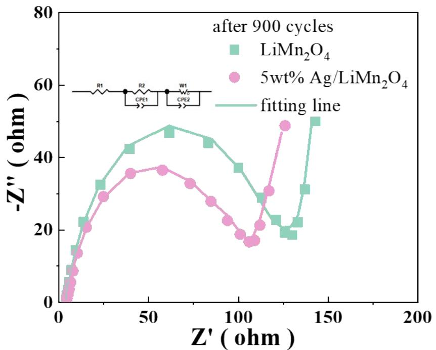
**Fig. S3** Electrochemical impedance spectroscopy plots of  $\text{LiMn}_2\text{O}_4$  and  $5\text{wt\% Ag}/\text{LiMn}_2\text{O}_4$  after 900 cycles at 5 C, the inset in S2 is the equivalent circuit.
