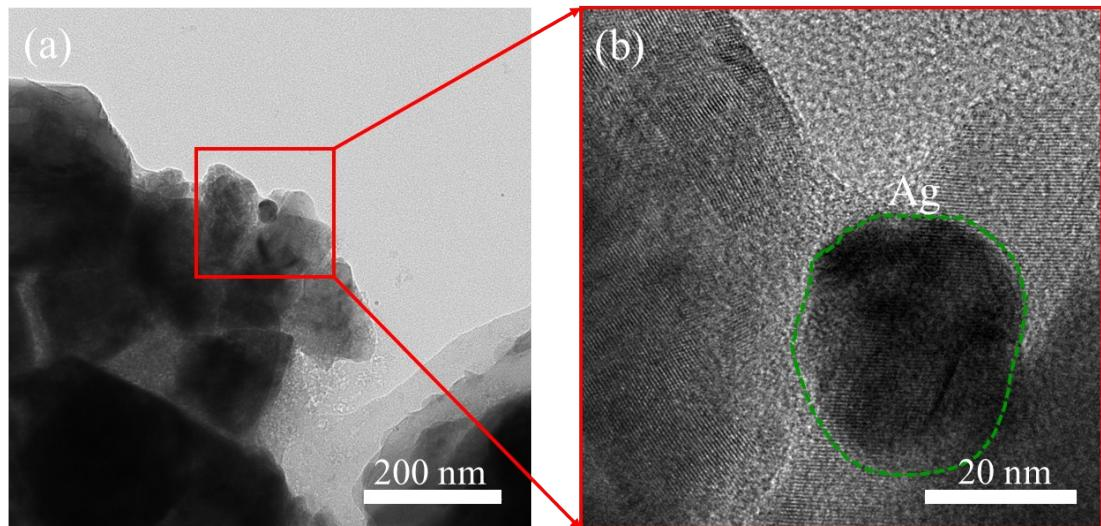
**Fig. S4** (a) TEM and (b) HR-TEM images of 5wt% Ag/LiMn<sub>2</sub>O<sub>4</sub> at 5 C after 900 cycles.
