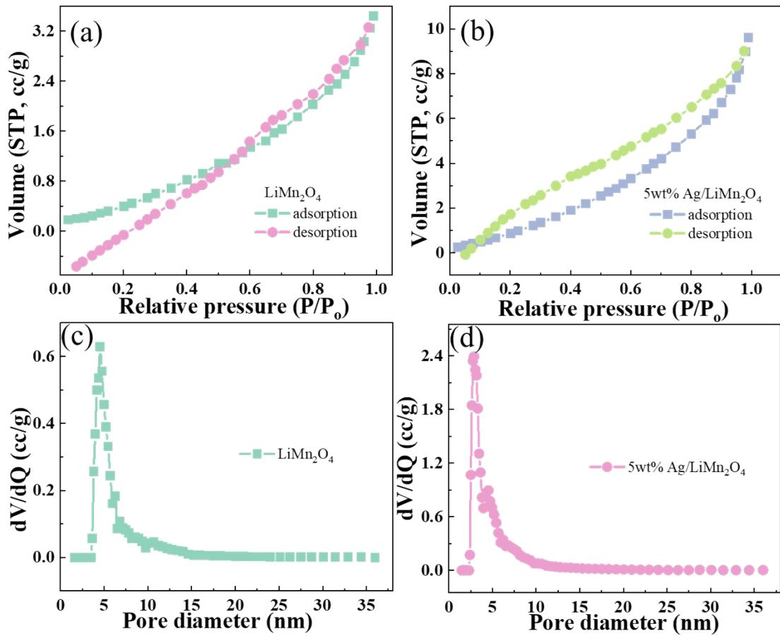
**Fig. S2** Nitrogen adsorption/desorption isotherms of the (a)  $\text{LiMn}_2\text{O}_4$  and (b) 5wt%  $\text{Ag}/\text{LiMn}_2\text{O}_4$  samples. The pore size of (c)  $\text{LiMn}_2\text{O}_4$  and (d) 5wt%  $\text{Ag}/\text{LiMn}_2\text{O}_4$  calculated from adsorption/desorption experiments using the BJH model.
