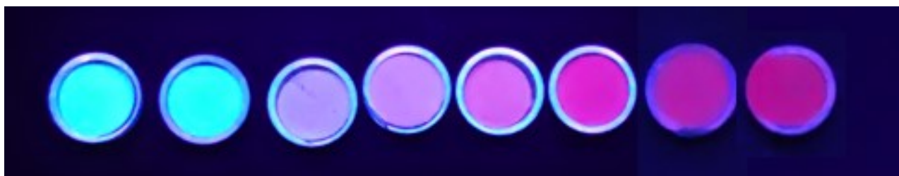
Fig. S6 The digital photographs of \text{CMZ}_{0.2}\text{GO}:\text{Bi}^{3+}/y\text{Mn}^{4+} ( y = 0, 0.001, 0.01, 0.02, 0.05, 0.08, 0.10, 0.15 ) under 365 nm light irradiation.
