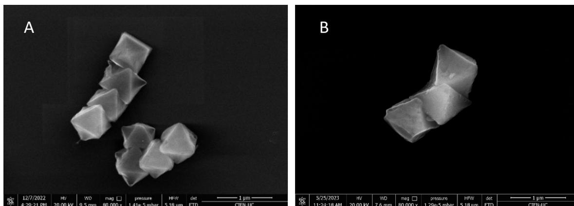
**Figure S6.** SEM images of MOF-808-M materials. MOF-808-Zr (A) and MOF-808-Hf (B) with a magnitude of 80,000.
