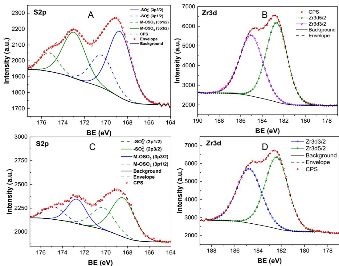
**Figure S8.** XPS corresponding to MOF-808-SO<sub>4</sub>-Zr before catalysis (A-B) and after catalysis (C-D).
