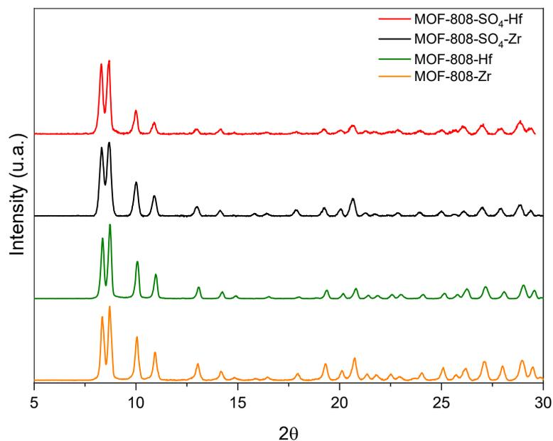
**Figure S13.** Powder X-ray diffraction patterns of MOF-808-SO<sub>4</sub>-Zr and MOF-808-SO<sub>4</sub>-Hf compared with its precursors.
