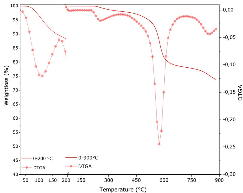
**Figure S12.** TGA MOF-808-SO<sub>4</sub>-Hf from 0-200 °C (left) and 0-900 °C (right).
