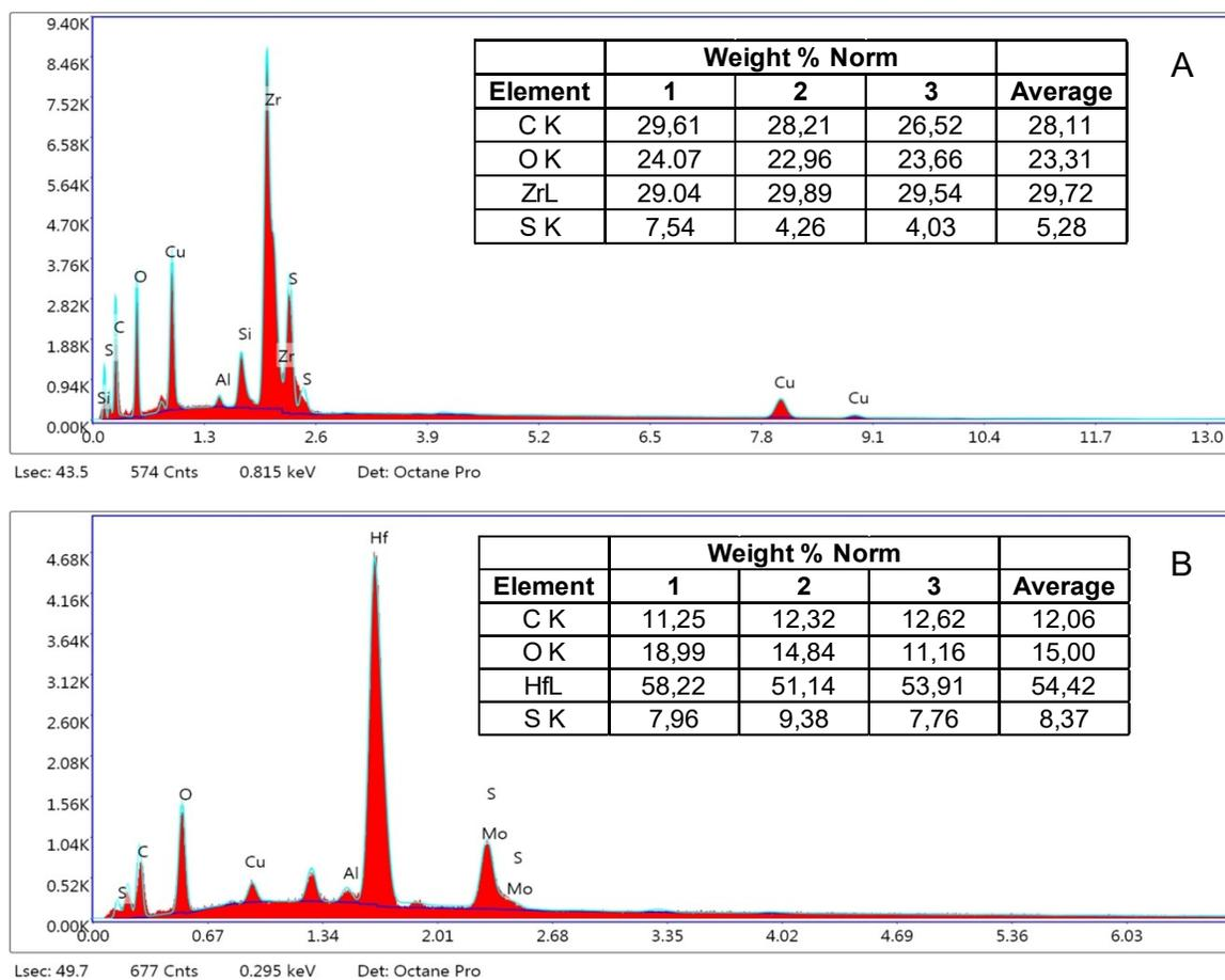
**Figure S7.** EDS for the materials MOF-808-SO<sub>4</sub>-Zr (A) and MOF-808-SO<sub>4</sub>-Hf (B).
