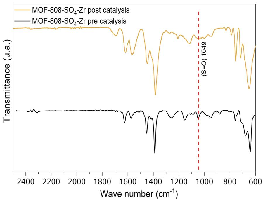
**Figure S10.** FT-IR of fresh MOF-808-SO<sub>4</sub>-Zr (black color) and MOF-808-SO<sub>4</sub>-Zr recovered after catalytic cycles (brown color).
