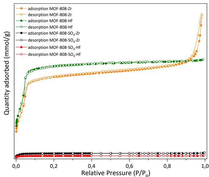
**Figure S4.** N<sub>2</sub> adsorption and desorption isotherm of MOF-808-SO<sub>4</sub>-Zr and MOF-808-SO<sub>4</sub>-Hf compared with their precursors.
