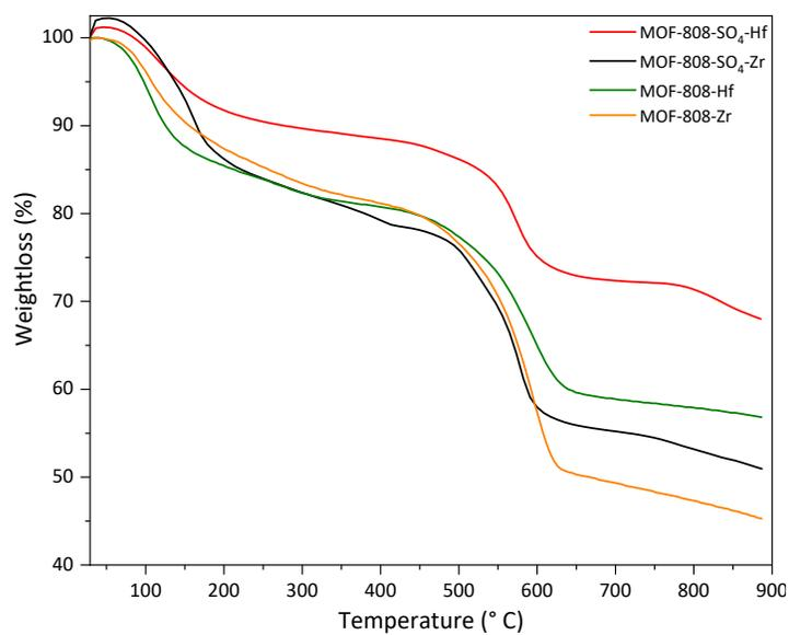
**Figure S5.** Thermogravimetric analysis of MOF-808-SO<sub>4</sub>-Zr and MOF-808-SO<sub>4</sub>-Hf compared with their precursors.
