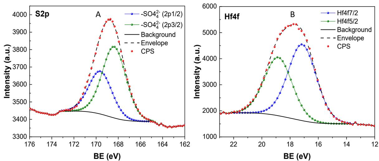
**Figure S9.** XPS corresponding to MOF-808-SO<sub>4</sub>-Hf before catalysis (A-B).
