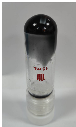
Figure S11. Polymerization of styrene and dibenzyl ether catalyzed by \text{MoO}_2 . Reaction conditions: \text{MoO}_2 100 mg, dibenzyl ether 0.1 mmol, dodecane 2.0 mL, 140 °C, Ar 1 atm.
