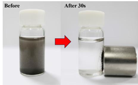
Fig. S5. Photo images of the MSS@MoS<sub>2</sub>-50 suspension before and after magnetic separation
