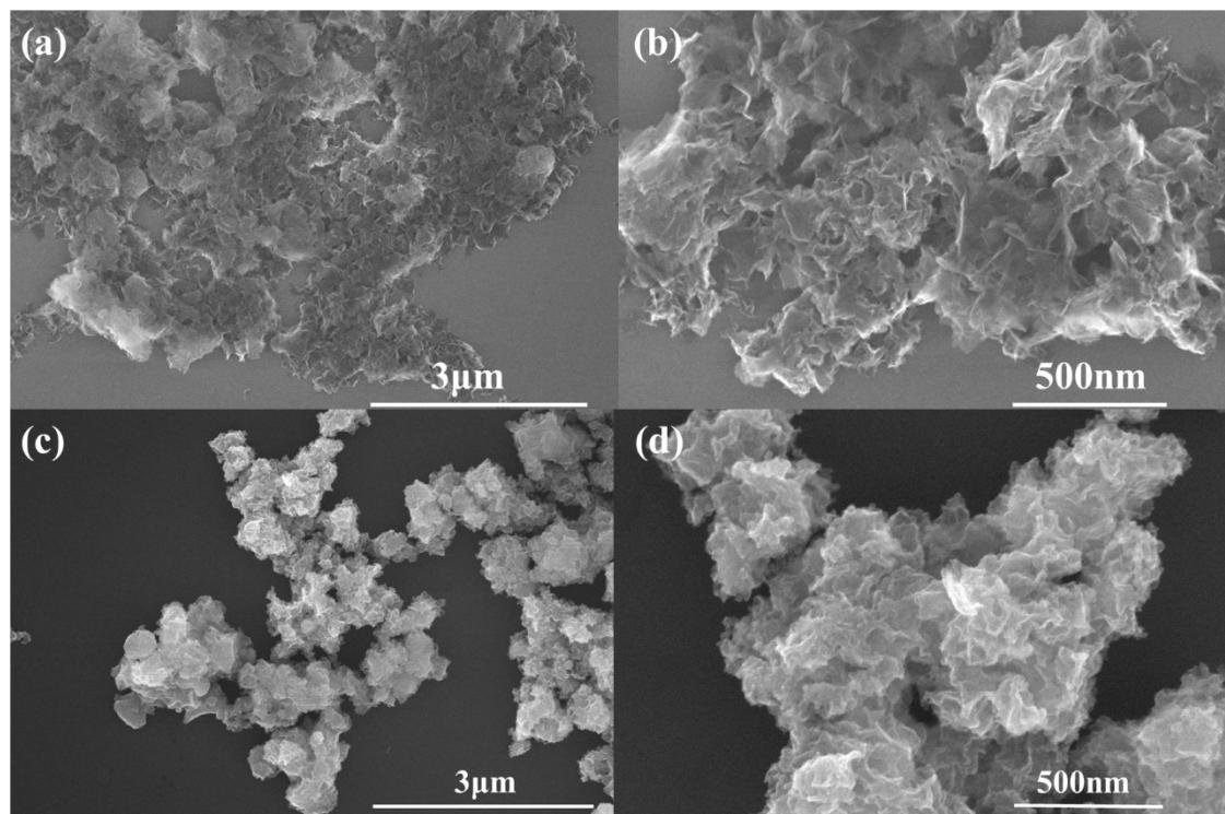
**Fig. S3** (a,b) SEM images of CoFe-LDH, and (c,d) SEM images of CoFeSe.
