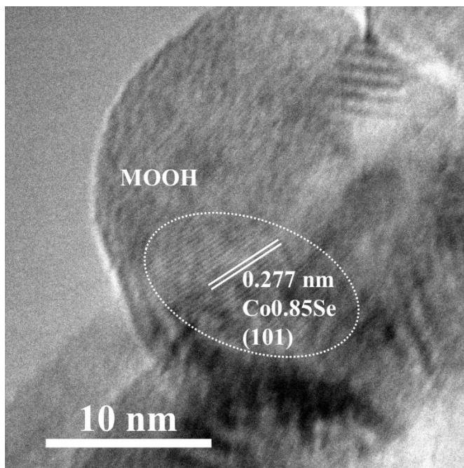
**Fig. S12** HRTEM image of CoNiFeSe after stability test.
