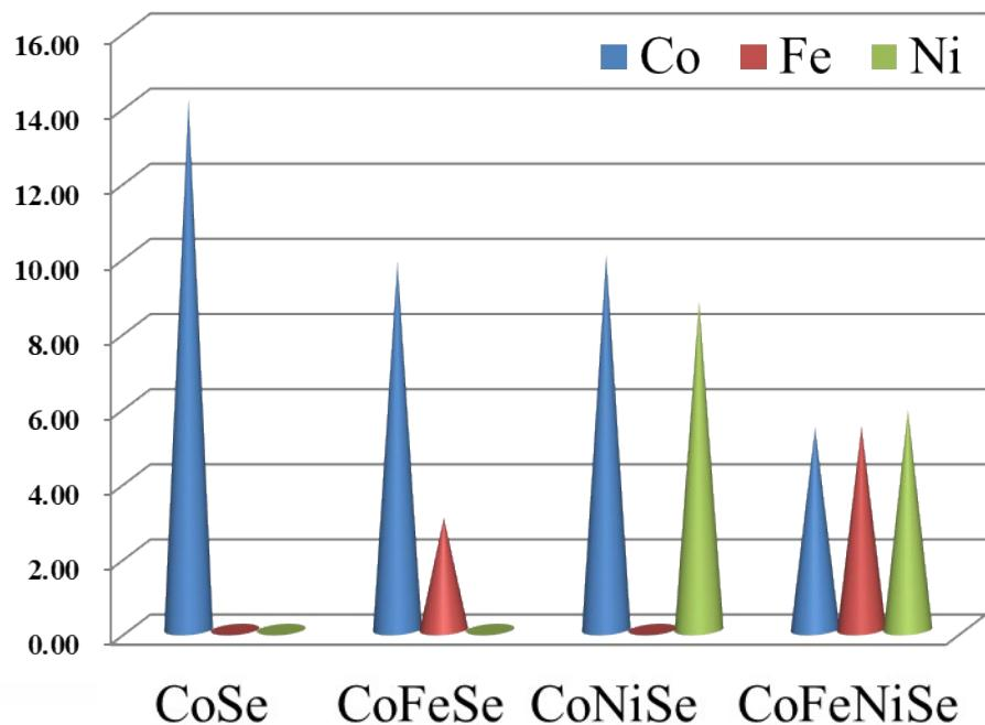
**Fig. S5** Atomic ratio of CoSe, CoNiSe, CoFeSe and CoNiFeSe.
