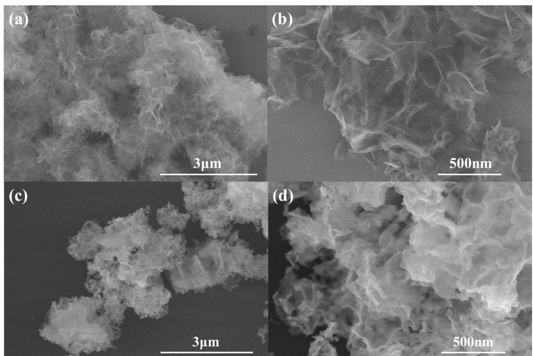
**Fig. S2** (a,b) SEM images of Co-LDH, and (c,d) SEM images of CoSe.
