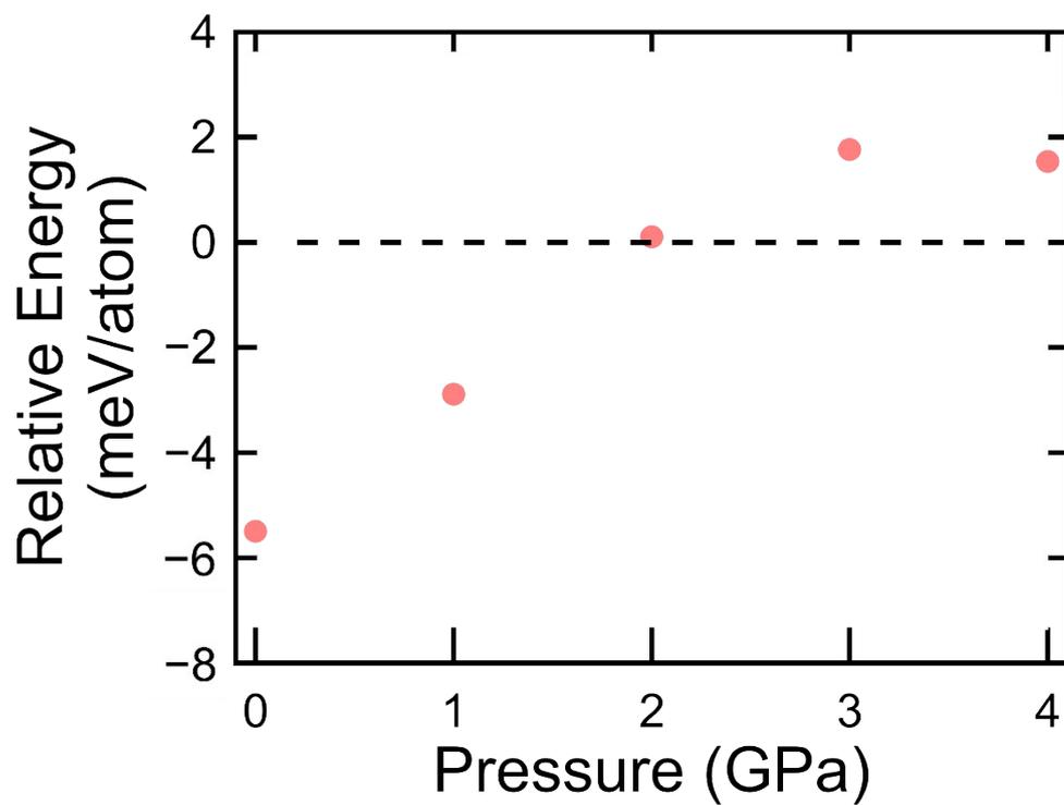
**Figure S3:** Relative energy of the SmSI-type structure compared to the Srl<sub>2</sub>-type structure in CeSI as a function of pressure. The most stable polymorph switches from SmSI-type to Srl<sub>2</sub>-type at 2 GPa.
