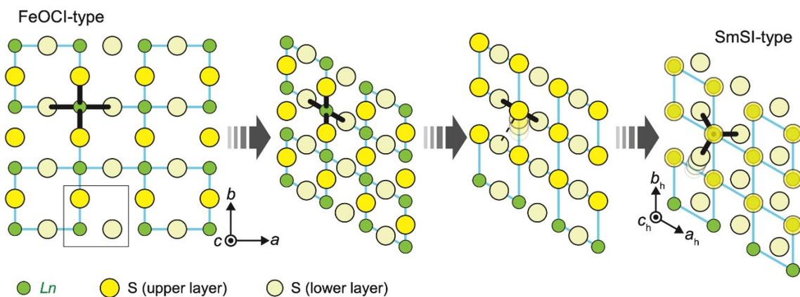
**Figure S2:** Schematic representation of the phase transition from the (left) FeOCl-type to (right) SmSI-type structures, and (middle) hypothetical sheared states. The stacking of upper S, lower S, and *Ln* layers along the *c* axis are illustrated from front to back. The black lines and blue diamonds represent the unit cell of the FeOCl- and SmSI-type structure, respectively.
