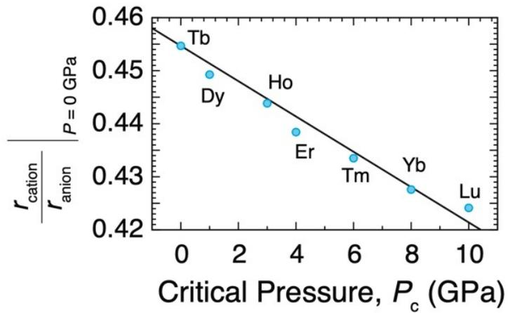
**Figure S4:** The cation-to-anion ratio (blue circles) calculated for Tb–Lu at ambient pressure as a function of critical pressure for transformation from FeOCl- to SmSI-type. The result of linear fitting is depicted by a black line.
