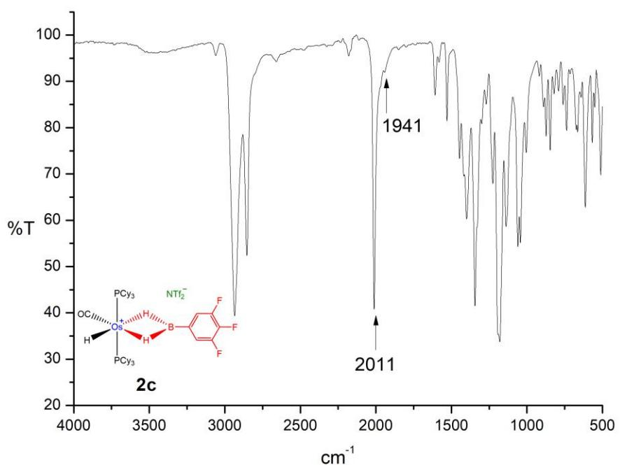
**Fig. S59** IR spectrum of **2c**.
