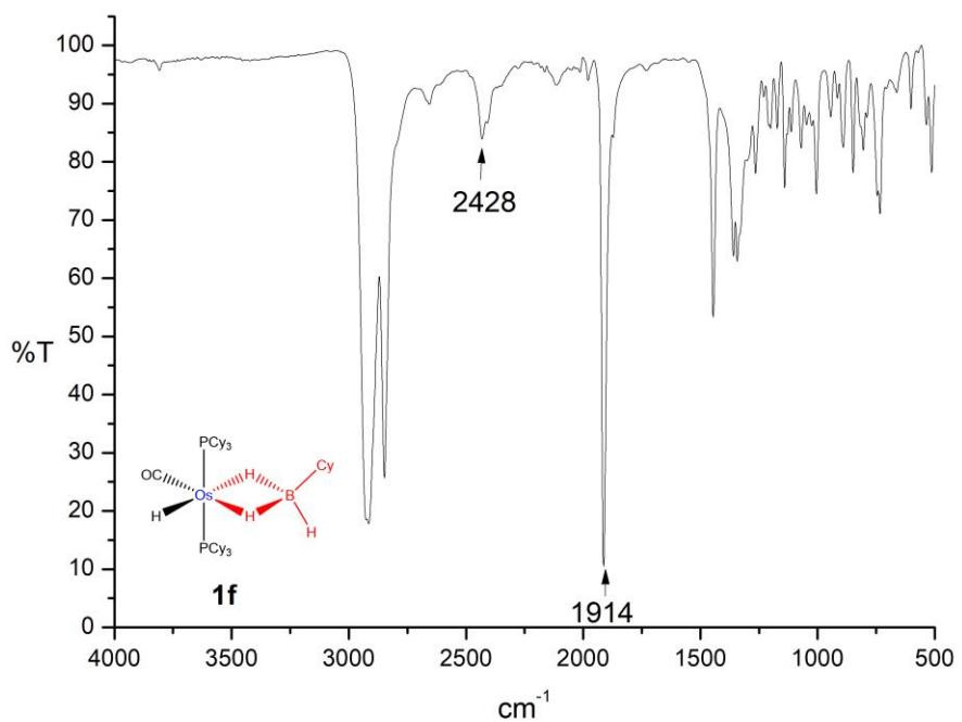
**Fig. S56** IR spectrum of **1f**.
