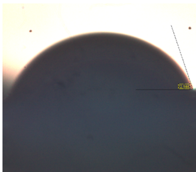
Figure S7. Representative contact angle measurement for Ce-TPTC-NH 2 MOF.
