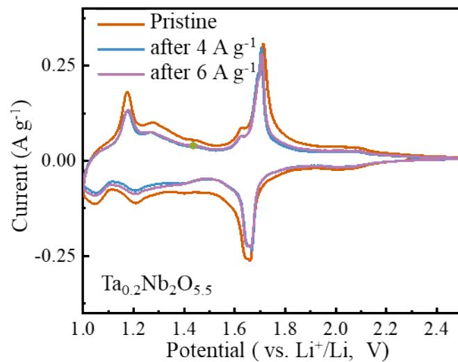
Figure S3. CV curves of  $\text{Ta}_{0.2}\text{Nb}_2\text{O}_{5.5}$  before and after cycling at different current densities at scan rate of  $0.1 \text{ mV s}^{-1}$ .
