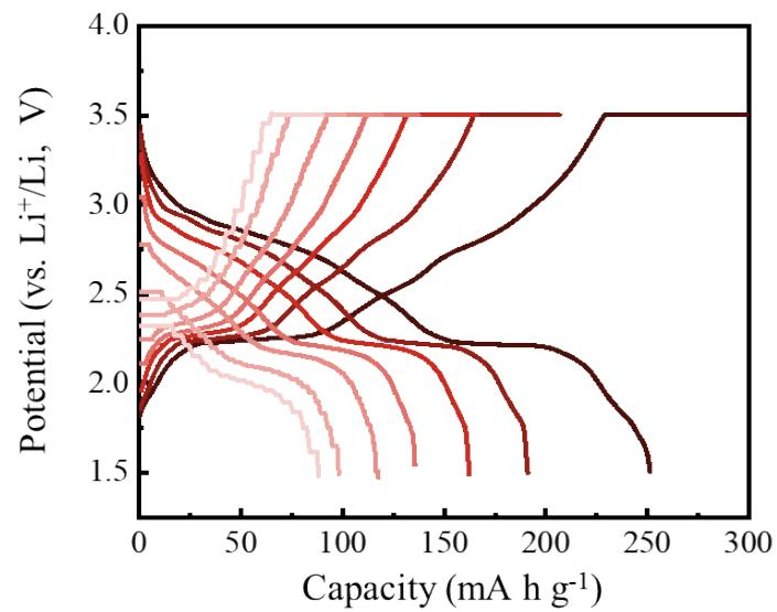
Figure S4. Charge-discharge voltage profiles of LCO/Nb<sub>2</sub>O<sub>5</sub> at 0.1, 0.2, 0.5, 1, 2, 4 and 6 A g<sup>-1</sup>.
