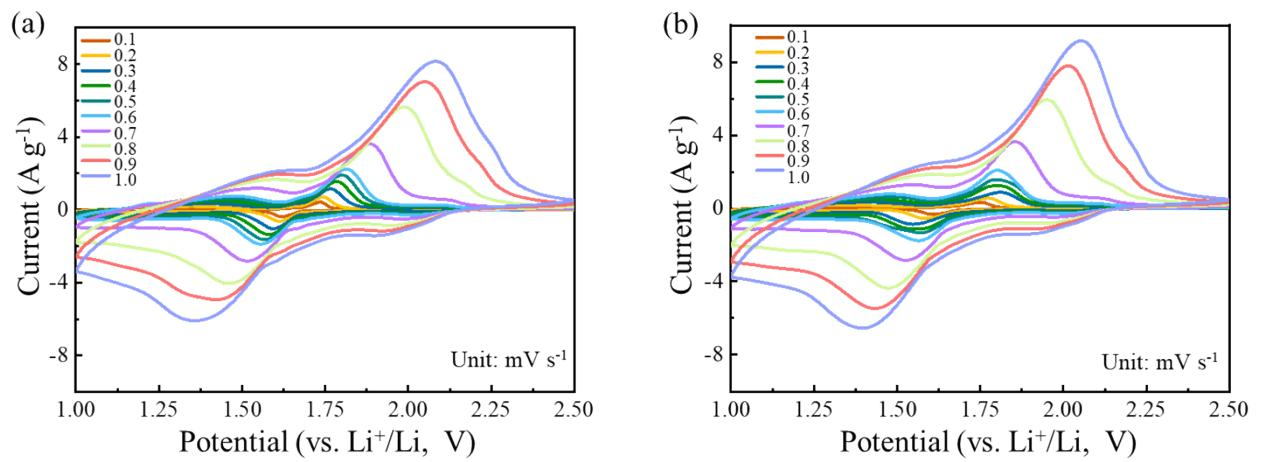
Figure S1. CV curves of  $\text{Nb}_2\text{O}_5$  (a) and  $\text{Ta}_{0.2}\text{Nb}_2\text{O}_{5.5}$  (b) at scan rate of 0.1 to 1.0  $\text{mV s}^{-1}$ .
