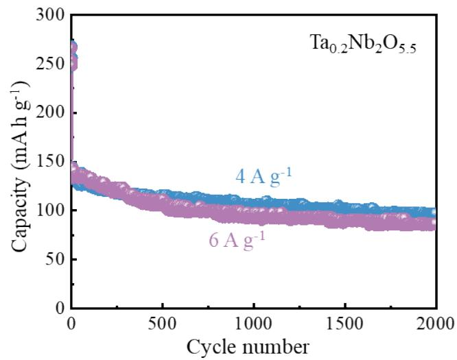
Figure S2. Cycling tests of  $\text{Ta}_{0.2}\text{Nb}_2\text{O}_{5.5}$  at  $4 \text{ A g}^{-1}$  and  $6 \text{ A g}^{-1}$ .
