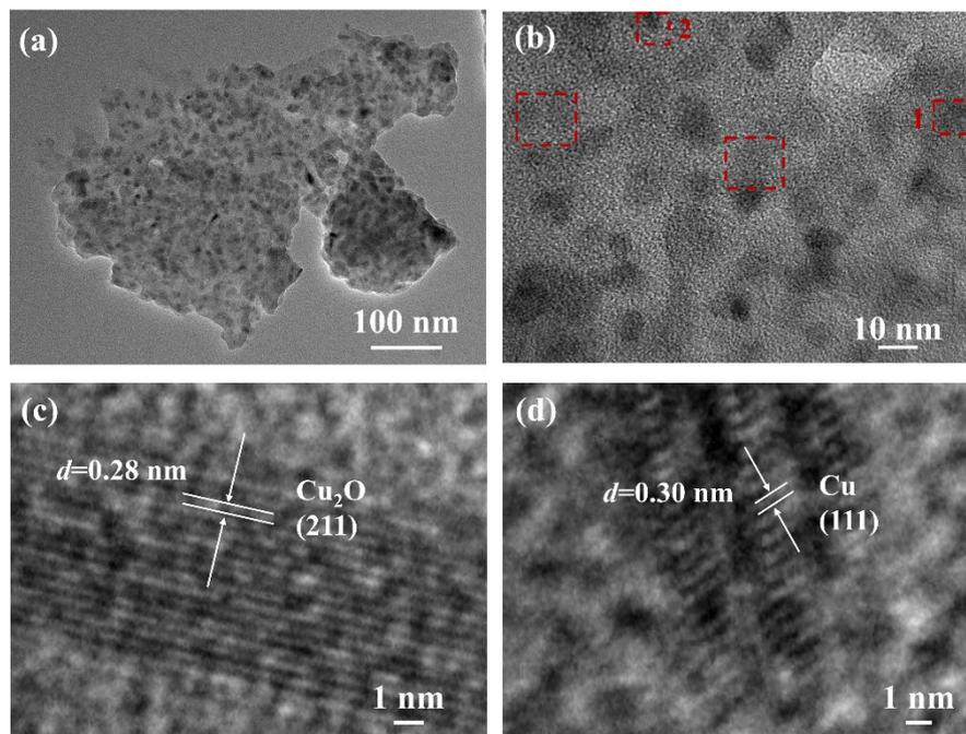
Figure S3 (a-b) The HR-TEM images of MOF-74/Cu<sub>2</sub>O/Cu; (c) the lattice spacing of selected area 1; (d) the lattice spacing of selected area 2
