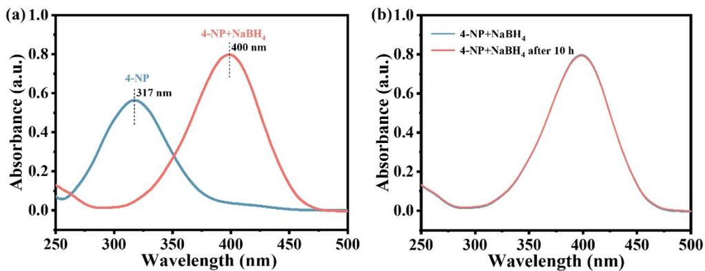
Figure S5 (a) The absorbance of 4-NP solution (blue line) and 4-NP solution with NaBH<sub>4</sub> (red line); (b) the absorbance of 4-NP solution with NaBH<sub>4</sub> (blue line) and standing for 10 h (red line)
