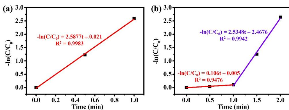
Figure S9 (a) Plot of  $-\ln(C/C_0)$  versus time for MOF-74/Cu<sub>2</sub>O/Cu; (b) Plot of  $-\ln(C/C_0)$  versus time for MOF-74
