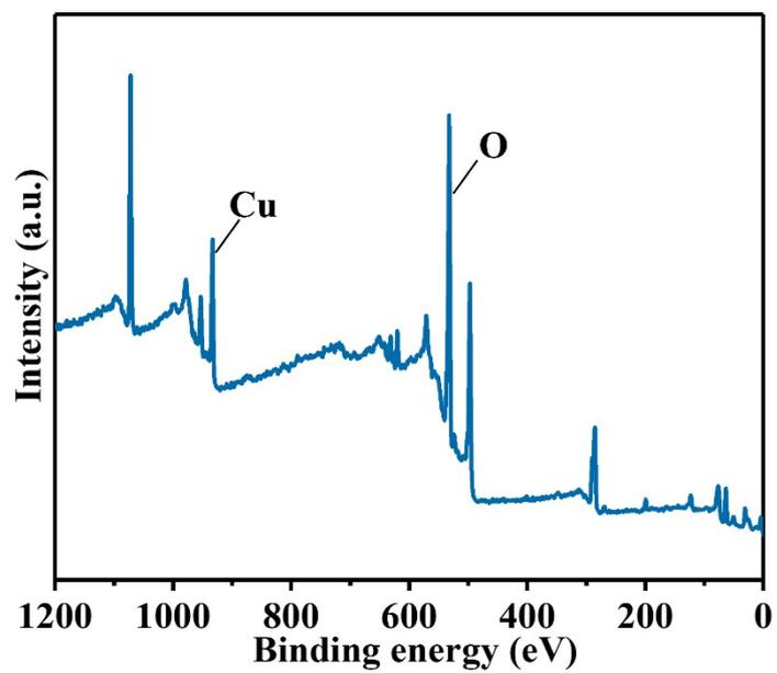
Figure S4. The XPS full spectrum of MOF-74/Cu<sub>2</sub>O/Cu
