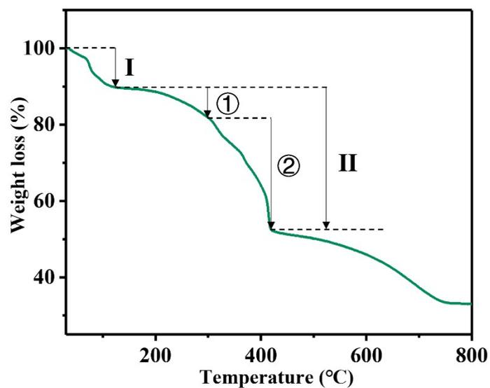
Figure S2 The TG of hierarchical MOF-74, I (25-150 °C): the desorption of solvent; II (200-400 °C): the decomposition of hierarchical MOF-74
