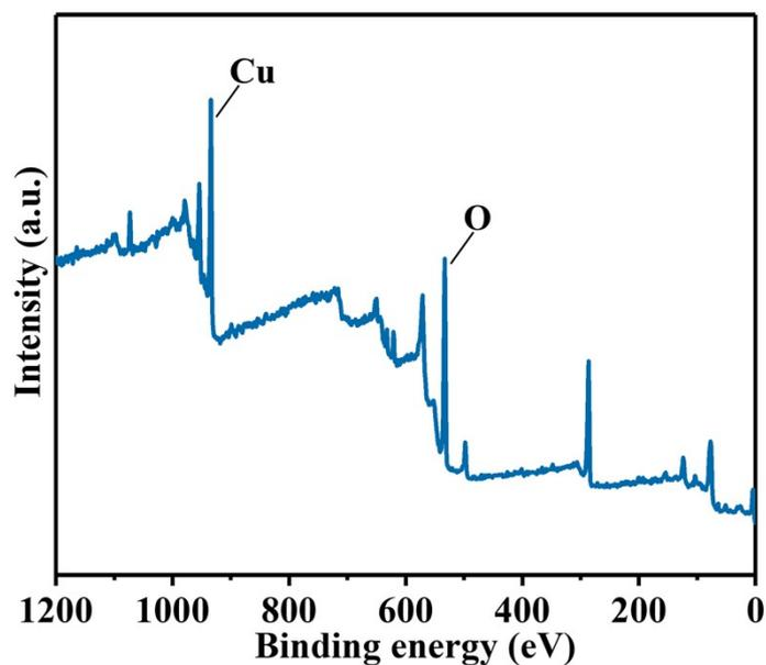
Figure S6. The XPS full spectrum of Cu<sub>2</sub>O/Cu
