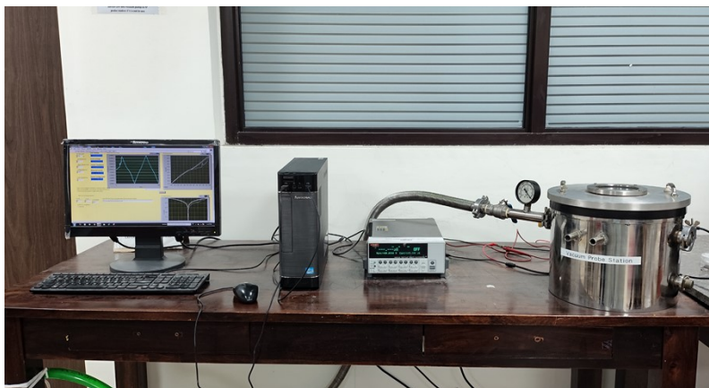
Figure S15: Vacuum probe station
