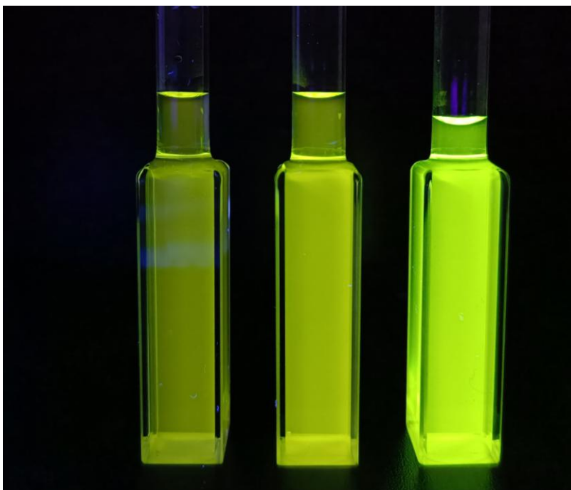
Figure S17. Photographs of MeCN solutions of complexes 1 , 2 and 3 (from left to right) at 2.5 \times 10^{-5} M concentration under UV irradiation at 298 K.
