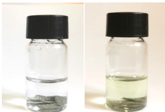
Fig. S1 Photographs of FU-NF in a capped bottle (left) before and (right) after the solvothermal process.
