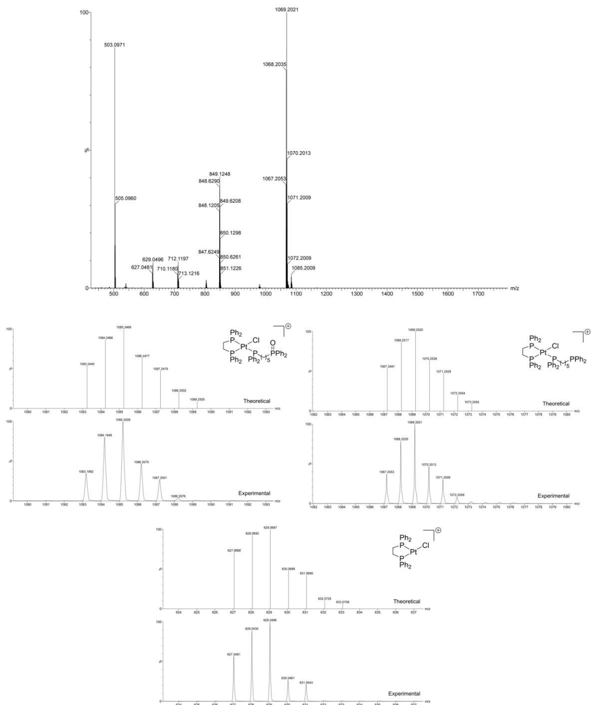
Fig. S159. Mass spectrum of Pt-2, including relevant fragments together with their respective theoretical isotope pattern
